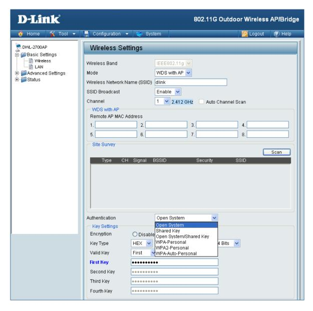
In WDS with AP mode, the DWL-2700AP wirelessly connects multiple networks, while still functioning as a wireless AP. WDS (Wireless Distribution System) allows access points to communicate with one another wirelessly in a standardized way. It can also simplify the network infrastructure by reducing the amount of cabling required. Basically the access points will act as a client and an access point at the same time.
