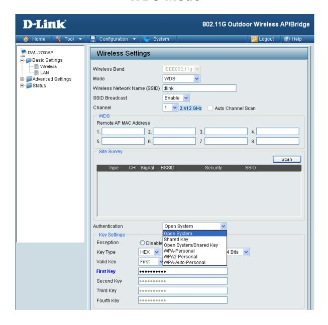
In WDS, the DWL-2700AP wirelessly connects multiple networks, without functioning as a wireless AP.
