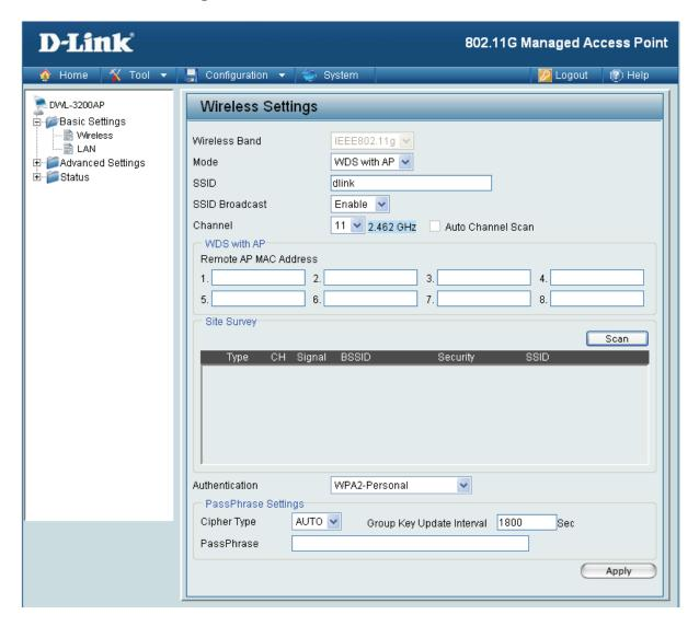
In WDS with AP mode, the DWL-3200AP wirelessly connects multiple networks, while still functioning as a wireless AP.
