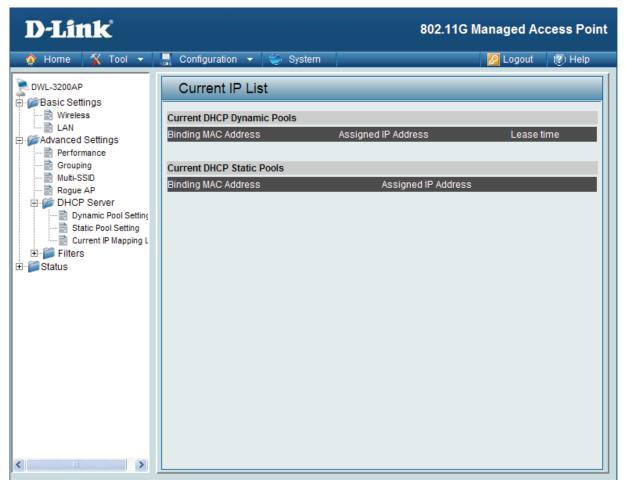
This screen displays information about the current DHCP dynamic and static IP address pools. This information is available when you enable the DHCP function of the DWL-3200AP and assign dynamic and static IP address pools.
