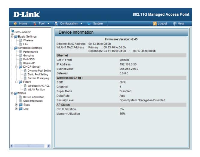
**Device Information:** This window displays the configuration settings of the DWL-3200AP, including the firmware version and device MAC address.
