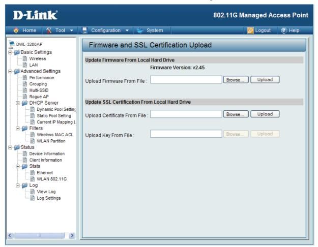
**Upload Firmware** After downloading the most recent version of firmware for the DWL-3200AP from http://support.dlink.com to your local computer, use the **Browse** button to locate the firmware file on your computer. Click **Upload** to update the firmware version.
