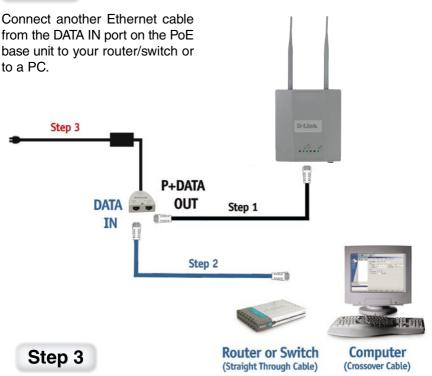
Attach the power adapter to the connector labeled POWER IN on the PoE base unit. Attach the power cord to the power adapter and into an electrical outlet.
