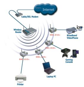
Connecting Ethernet Devices to a Wireless Network
