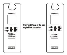
When using a DMC-920R that the TX(transmit) is  $1310\mu$ m and the RX(receive) is  $1550\mu$ m, then the other end need to have a combination of DMC-920T that the TX(transmit) is  $1310\mu$ m and the RX(receive) is  $1550\mu$ m.
