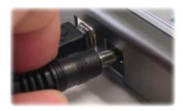
Plug the USB type B connector (the smaller end of the cable) into the back of the DUB-H7.
