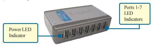
Note: If a port becomes overloaded, a "current exceeded" event will take place. The LED of the port will turn off and the message "USB HUB Current Limit Exceeded" appears on the monitor. Reset the DUB-H7 by disconnecting it for 5 seconds and then powering it back on by connecting the AC power adapter.
