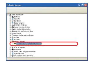
Look under **Device Status** to check that the device is working properly. Click **OK** to continue.
