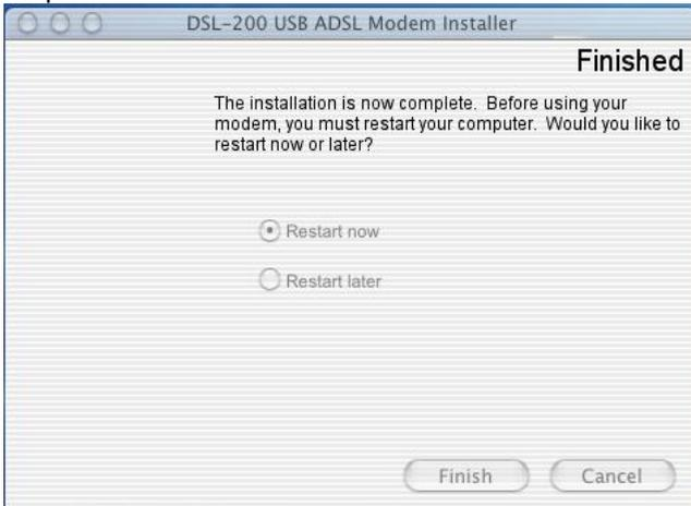
6. The USB driver is now installed. Before using your USB ADSL modem, connect the modem to the computer using the proper USB device cable and connect the DSL line to the USB ADSL modem.
