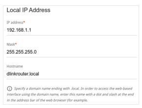
Figure 85. Configuring the local interface. The IPv4 tab. The Local IP Address section.
