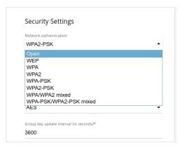
Figure 95. Network authentication types supported by the router.
