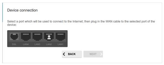
Figure 35. The page for configuring a LAN port as the WAN port.
