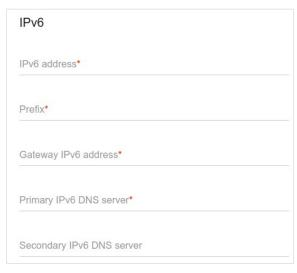
Figure 65. The page for creating a new **Static IPv6** connection. The **IPv6** section.
