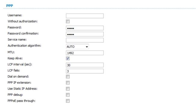
Figure 55. The page for creating a new connection. The **PPP** section.
