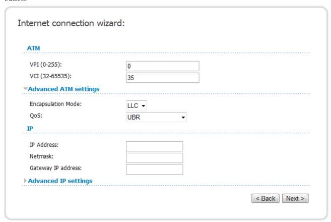
Figure 30. Configuring Static IP WAN connection.
