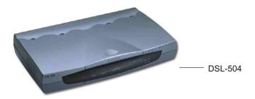
This remote router features 1 ADSL WAN port, 4 10/100Mbps switched LAN ports, IP routing, transparent bridging, NAT/DHCPInternet gateway functions and VPN.
