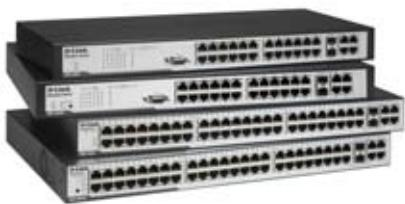
DES-3028 / DES-3052 Series provides flexible choices of 24 or 48 Fast Ethernet ports, with or without Power over Ethernet. Each switch is equipped with four Gigabit Ethernet ports including two combo SFP which are capable of both Gigabit and Fast Ethernet (100BASE-FX) fiber connections for user-specific applications.
