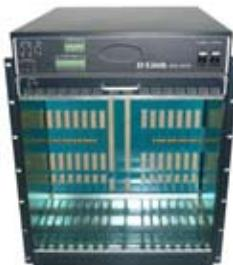
The IP DSL Access Multiplexers (DSLAMs) are carrier-class, high performance devices deployed at the service provider CO (central office) side. They provide IP-based broadband access services to ADSL subscribers CPE (consumer premise equipment) in the multi-unit, multi-tenant buildings over the existing telephone line.
