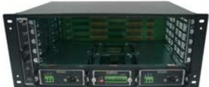
The IP DSL Access Multiplexers (DSLAMs) are carrier-class, high performance devices deployed at the service provider CO (central office) side. They provide IP-based broadband access services to ADSL subscribers CPE (consumer premise equipment) in the multi-unit, multi-tenant buildings over the existing telephone line.
