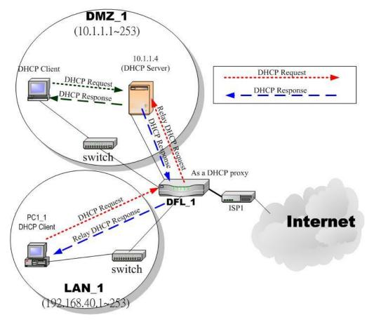
Figure 4-3 DHCP Relay mechanism chart
