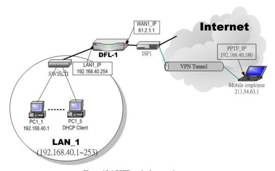
Figure 15-1 PPTP method connection
