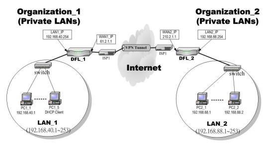
Figure 11-1 Organization 1 LAN 1 is making VPN tunnel with Organization 2 LAN 2
