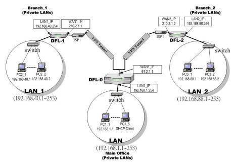
Figure 14-2 The Topology of the VPN Hub (Main Office) and VPN Spoke (Branch offices)
