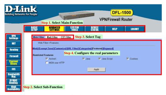
Figure 2-2 You can select the functional area by the sequence in Web GUI
