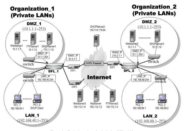
Figure 2-1 Typical topology for deploying DFL-1500
