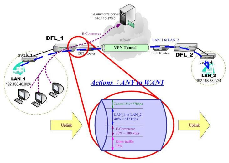
Figure 21-2 Use bandwidth management mechanism to shape the data flow on the uplink direction
