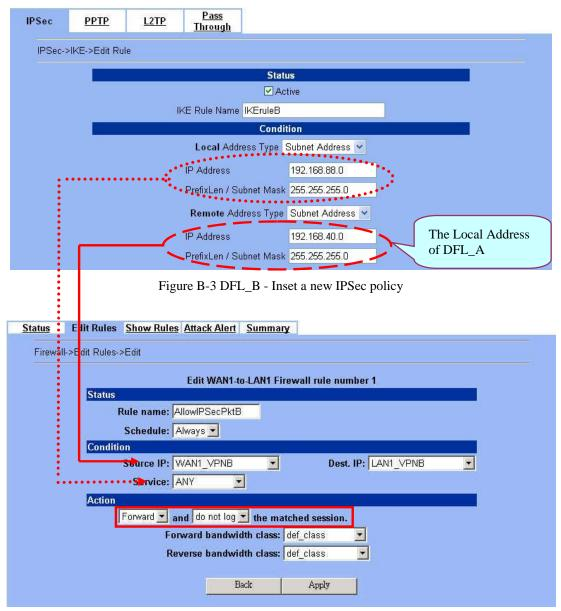
Figure B-4 DFL\_B - Insert a new firewall rule in WAN to LAN
