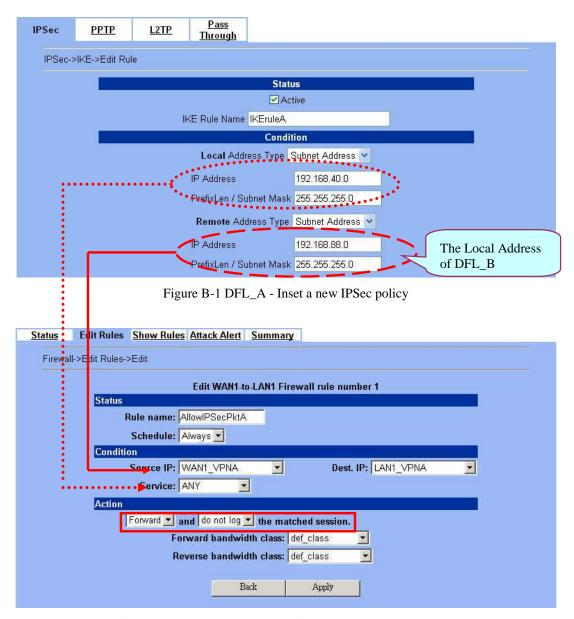
Figure B-2 DFL\_A - Insert a new firewall rule in WAN to LAN
