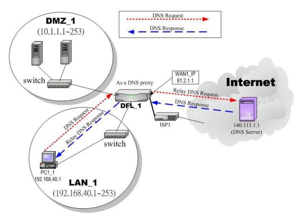
Figure 4-2 DNS Proxy mechanism chart
