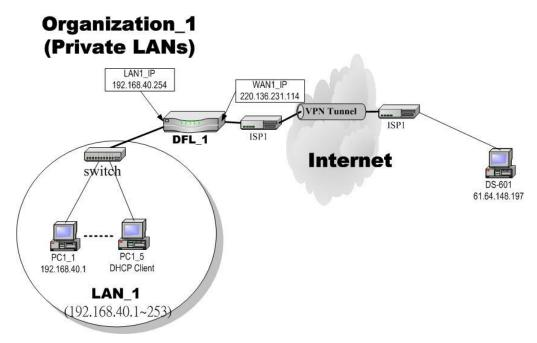
Figure 13-1 The client DS-601 is making IPSec VPN tunnel with Organization\_1 LAN\_1
