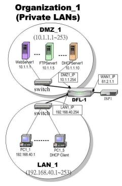
Figure 7-1 All the internal PCs can connect internet through limited WAN IP address by using NAT technology
