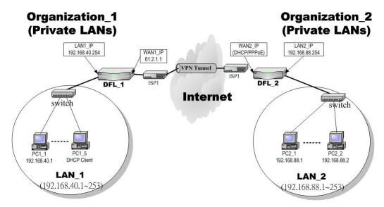
Figure 12-1 Organization 1 LAN 1 is making dynamic VPN tunnel with Organization 2 LAN 2
