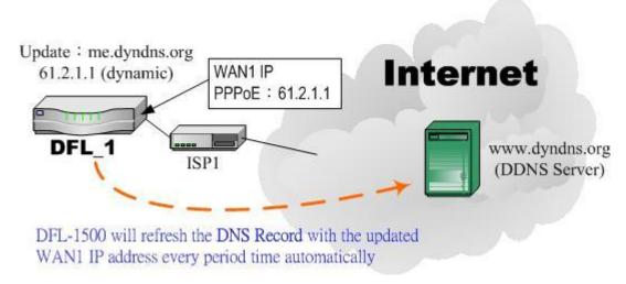
Figure 4-1 DDNS mechanism chart
