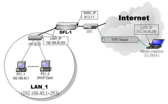
Figure 16-1 L2TP method connection
