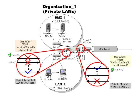
Figure 9-1 Setting up the firewall rule
