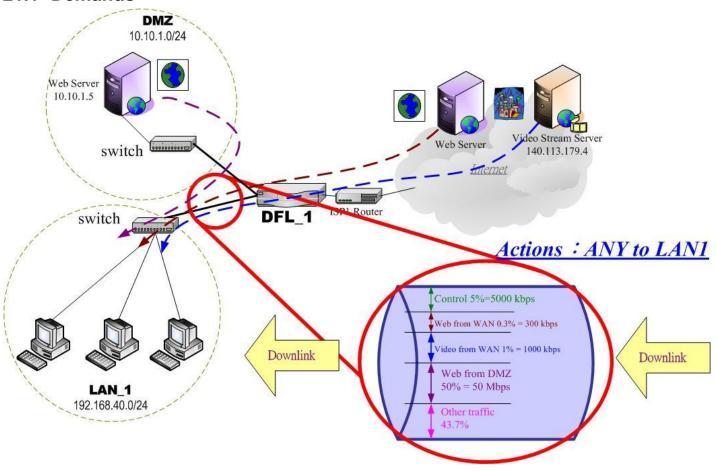
Figure 21-1 Use bandwidth management mechanism to shape the data flow on the downlink direction
