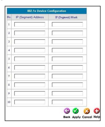
802.1x is a standard for passing the Extensible Authentication Protocol (EAP) packets over a LAN. You should enable this if there are any 802.1x devices between the DFL-600 and the RADIUS server on the WAN.
