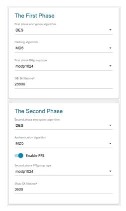
Figure 120. The page for adding an IPsec tunnel. The First Phase / The Second Phase sections.
