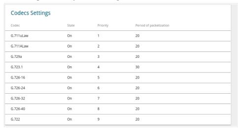
Figure 128. The VolP / Audio Settings page. The Codecs Settings section.
