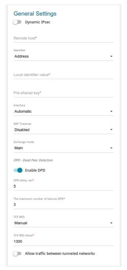
Figure 119. The page for adding an IPsec tunnel. The **General Settings** section.
