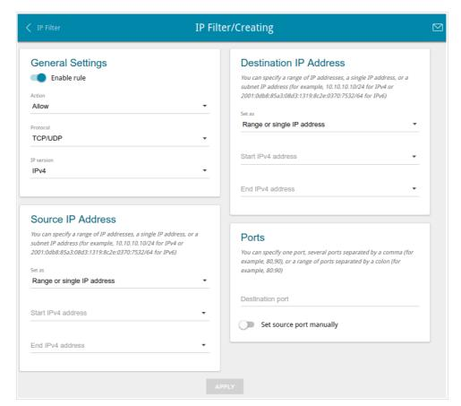
Figure 137. The page for adding a rule for IP filtering.
