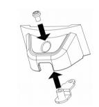
Slide the cover over the cable ports.
