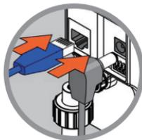
Connect the other end of the Ethernet cable to your D-Link Cloud Router and connect the camera's power adapter to a power outlet.
