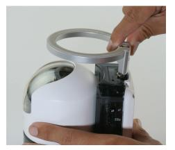
Tighten the nut on the top of the mounting stand using a coin or a screwdriver.
