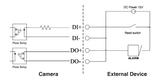
As the Digital Input signal is controlled by an external device, we recommend that you set your device to feed no current normally, and feed a 12V current only to trigger a DI event on the DCS-5605/5635.
