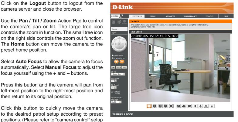
Pan Speed: This setting changes the camera's pan speed. The slowest value is 1 while fastest value is 10.
