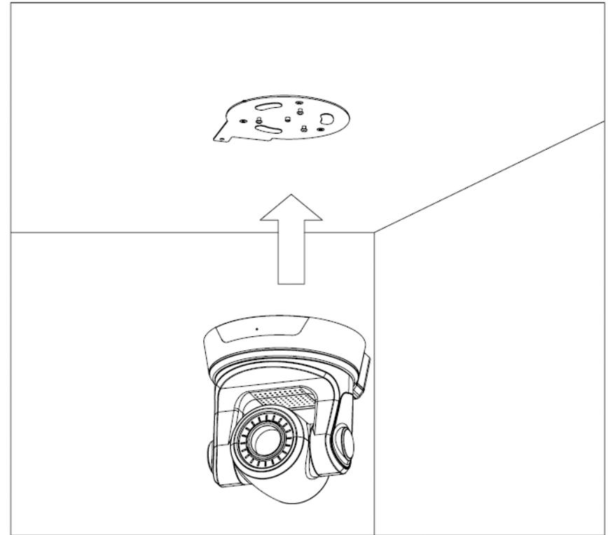
3. Rotate the base of the camera to lock it onto the bracket.
