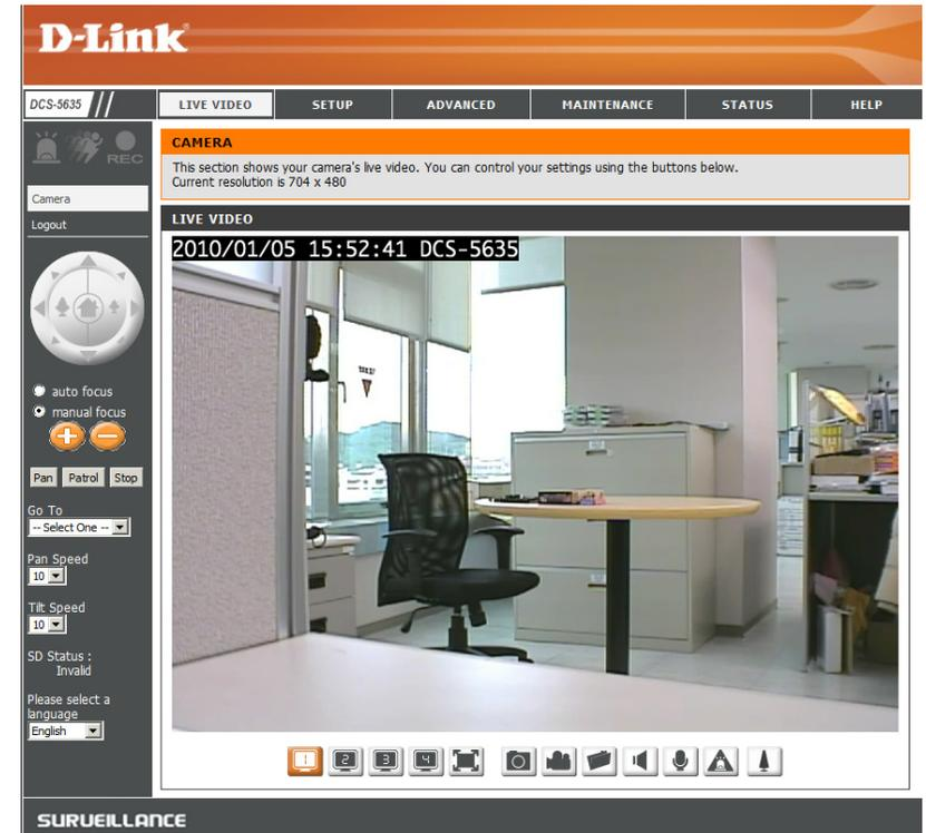
**Pan Speed:** This setting changes the camera's pan speed. The slowest value is 1 while fastest value is 10.
