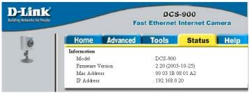
The Information table provides detailed information about the DCS-900 such as the Model Name, Firmware Version, Mac Address, and IP Address.
