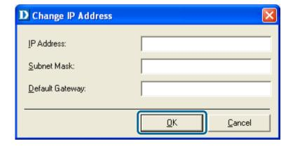
Enter the new **IP Address**, the **Subnet Mask** and the **Default gateway** into the respective fields and click **OK.** IPView Lite will apply the new IP Address to the camera.
