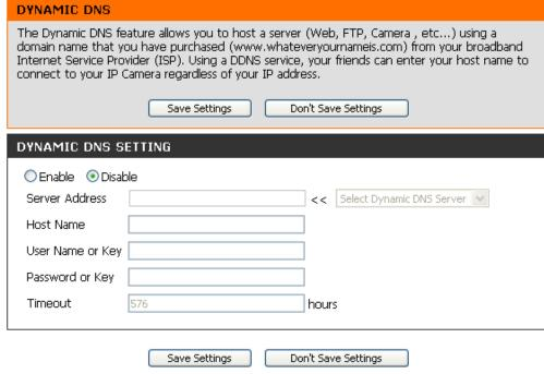
**DDNS:** (Dynamic Domain Name Server) will hold a DNS host name and synchronize the public IP address of the modem when it has been modified. The username and password are required when using the DDNS service.
