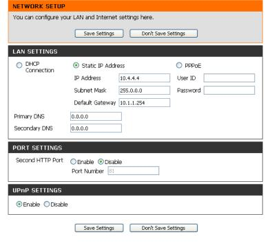
Port Settings: You may configure a Second HTTP port that will allow you to connect to the camera via a standard web browser. The port can be set to a number other than the default TCP ports 80. A corresponding port must be opened on the router. For example, if the port is changed to 1010, users must type in the web browser "http://192.168.0.100:1010" instead of "http://192.168.0.100".
