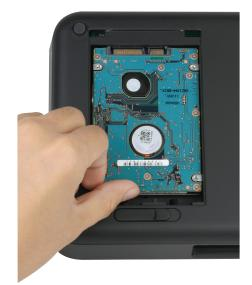
Place the bracket over the hard drive as shown, and secure the hard drive with the included screws. Replace the hard drive cover and slide the drive lock to the locked position.
