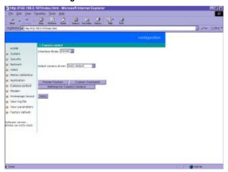
Since Video Server can be used in either Ethernet network or PPP network, the single serial port can be used to control either external COM port devices like a PTZ camera or modem. While in PPP interface, go to Modem page for modem configuration. Options on this page will be ignored.
