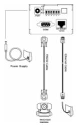
Shut down all the peripheral devices prior to connection. Connect the supplied cables from Video Server to related devices according to the following steps. Note that the power adaptor must be kept unplugged until other cables are firmly connected.
