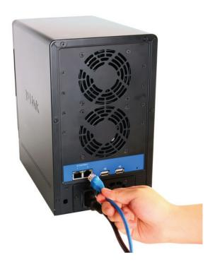
6. Connect the supplied power adapter to the power receptacle.
