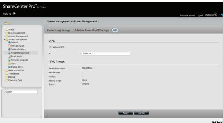
A network UPS slave communicates with network UPS master to receive the UPS status. To set up your NAS with UPS as network slave mode, follow the steps below:
