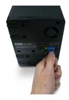
Finally, connect the supplied power adapter to the power receptacle on the back of the device.
