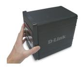
Once the faceplate is unlatched, pull it off of the device, exposing the drive bays.
