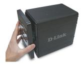
Insert a 3.5" SATA hard drive into an available drive bay. Make sure to align the drive connector to the endpoint in the DNS-343. Gently push the drive in until it connects. Repeat for each drive you are placing in the DNS-323.
