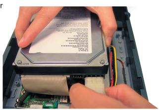
**D.** Use the mounting screw to secure the hard drive to the DSM-G600.
