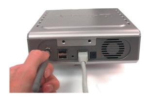
H. Connect the power adapter to the connector on the back panel of the DSM-G600. Then plug the other end of the power adapter into a wall outlet or power strip. After pressing the Power button, the Power LED will come on to indicate proper operation.
