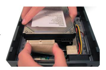
**C.** Connect the power cable to the power connector on your hard drive.
