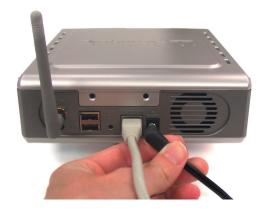
**Note:** When you first power on, the DSM-G600 will automatically format your hard drive if it is unformatted. This process may take several minutes depending on the size of your hard drive. During this process, the power LED will blink. Once the power LED is solid, you may then access the web-based configuration of the DSM-G600. Do not power the unit off during this process.
