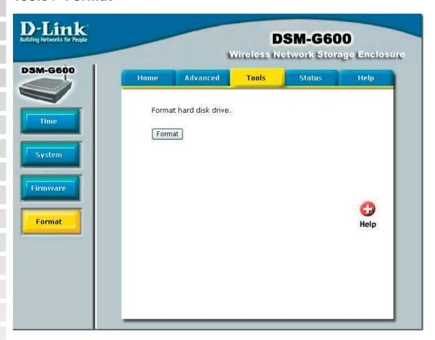
Before you can use the Internal hard drive, you must format it using the DSM-G600. If you install an unformatted hard drive, the DSM-G600 will automatically format the drive when the device is powered on for the first time.
