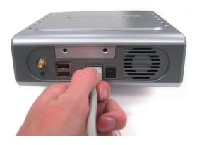
**Note:** It is required that an Ethernet cable is used during initial setup. Once your wireless configuration is set, you may disconnect the Ethernet cable and begin communicating wirelessly with your DSM-G600.
