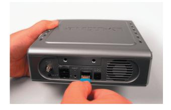
**Note:** It is required that an Ethernet cable is used during initial setup. Once your wireless configuration is set, you may disconnect the Ethernet cable and begin communicating wirelessly with your DSM-G600.
