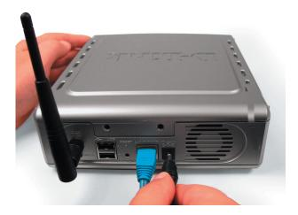
**Note:** When you first power on, the DSM-G600 will offer to format your hard drive if it is unformatted. This process may take several minutes depending on the size of your hard drive. During this process, the power LED will blink. Once the power LED is solid, you may then access the web based configuration of the DSM-G600. Do not power the unit off during this process.
