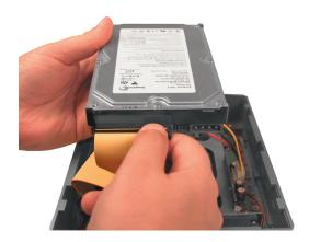
**C.** Connect the power cable to the power connector on your hard drive.
