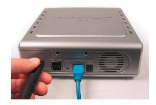
H. Connect the power adapter to the power receptor on the back panel. Then plug the other end of the power adapter into a wall outlet or power strip. The Power LED will turn on to indicate proper operation.
