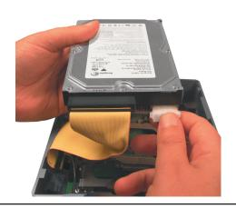
**D.** While facing the back of the DSM-G600, insert the right side of the hard drive into the case. Once in place, snap down the left side.
