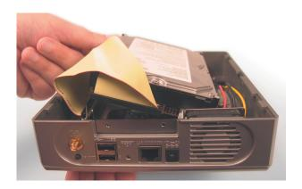
E. Use the mounting screw to secure the hard drive to the DSM-G600. Replace the cover and screw the two screws on the back panel of the DSM-G600.
