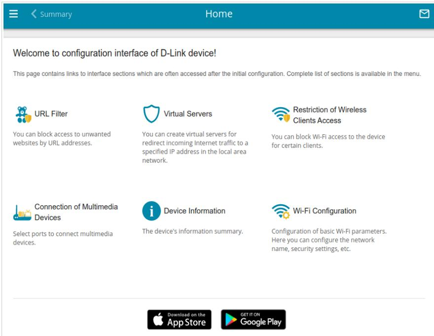
The web-based interface of the router is multilingual. You can select the needed language upon the initial configuration of the web-based interface of the router or in the **System / Configuration** section of the menu.
