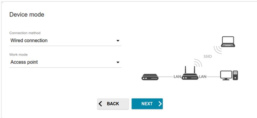
In order to connect your device to a wireless router for extending the range of the existing wireless network, on the **Device mode** page, from the **Connection method** list, select the **Wi-Fi** value. Then from the **Work mode** list select the **Repeater** value. In this mode you can change the LAN IP address, connect your device to another access point, set your own settings for the wireless network, and set your own password for access to the web-based interface of the device.
