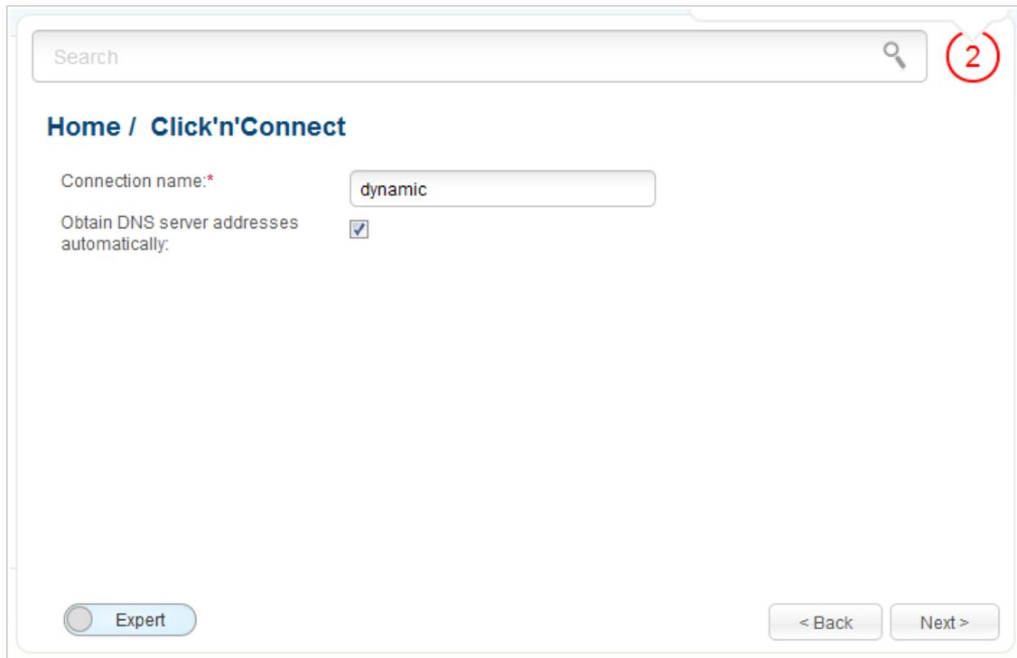
Figure 34. Configuring Dynamic IP WAN connection.
