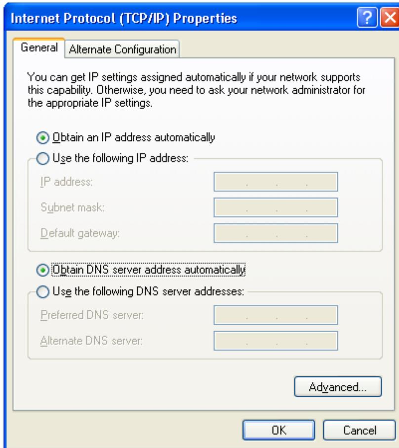
Figure 6. The **Internet Protocol (TCP/IP) Properties** window.
