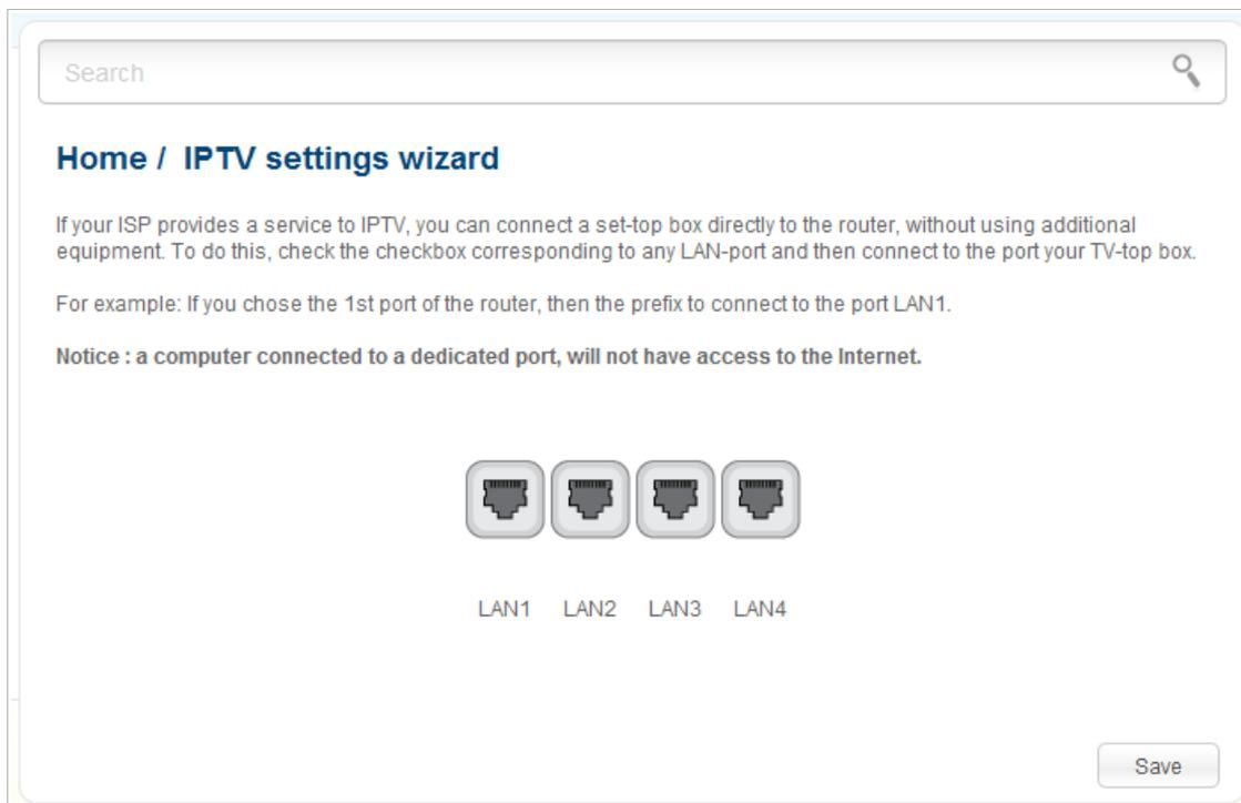
Figure 83. The page for selecting a LAN port to connect an IPTV set-top box.
