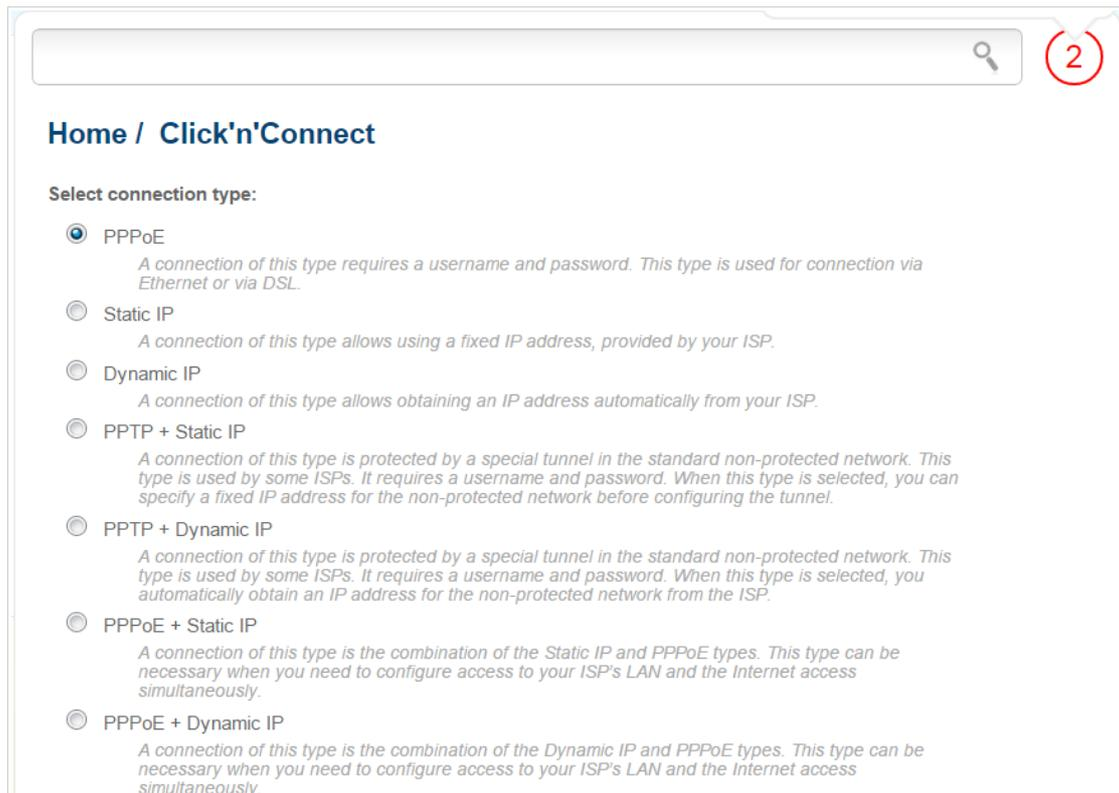
Figure 25. The page for selecting the connection type.
