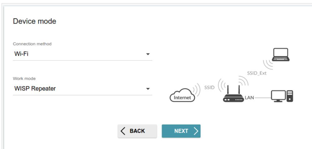
Figure 36. Selecting an operation mode. The **WISP Repeater** mode.
