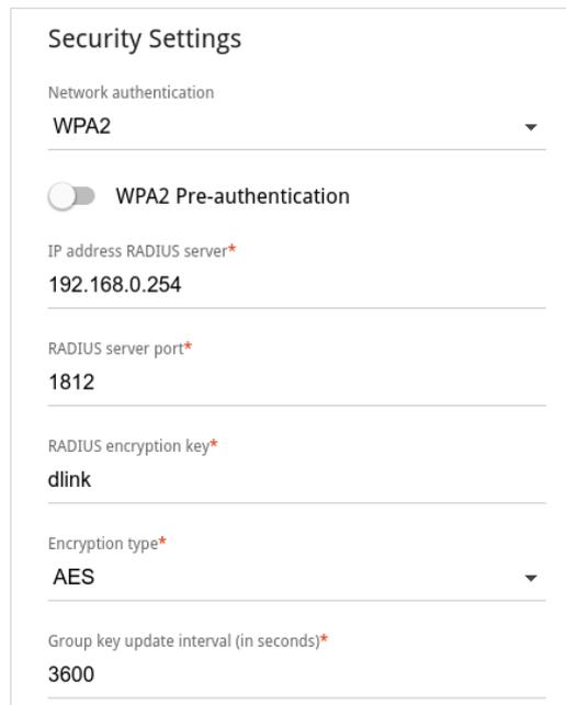
The screenshot shows the 'Security Settings' section of a web interface. It features a 'Network authentication' dropdown menu with 'WPA2' selected. Below this is a 'WPA2 Pre-authentication' toggle switch. There are five input fields: 'IP address RADIUS server\*' with the value '192.168.0.254', 'RADIUS server port\*' with '1812', 'RADIUS encryption key\*' with 'dlink', 'Encryption type\*' with 'AES', and 'Group key update interval (in seconds)\*' with '3600'.
