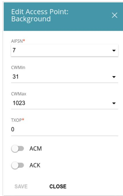
Figure 100. The window for changing parameters of the WMM function.
