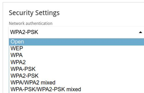
Figure 78. Network authentication types supported by the router.
