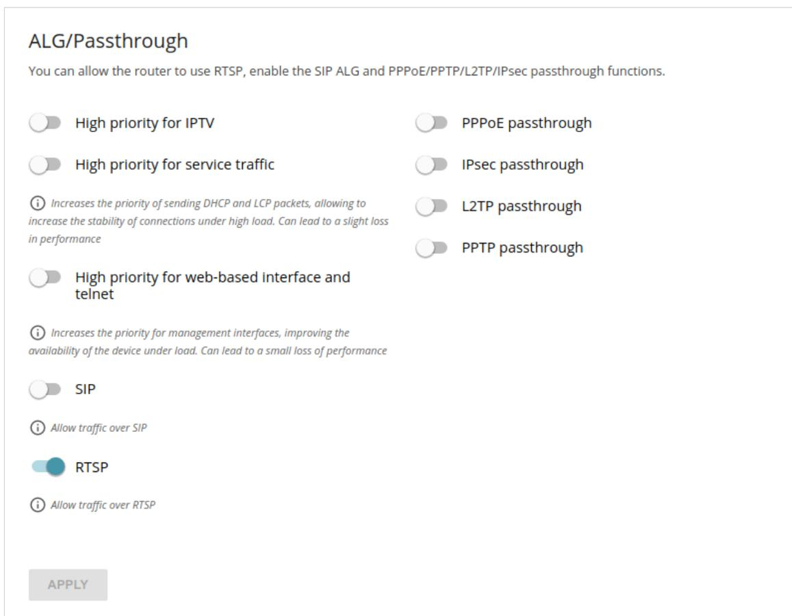
Figure 123. The **Functions / Advanced / ALG/Passthrough** page.
