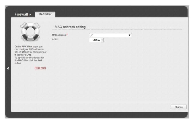
Figure 136. The page for adding an address for the MAC filter.
