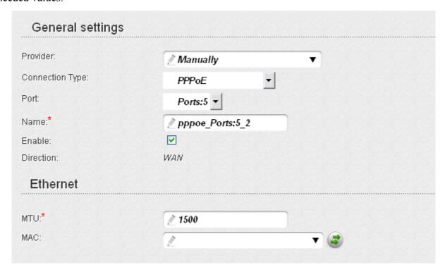
Figure 80. The page for creating a new connection. The **General settings** and **Ethernet** sections.
