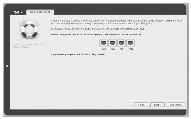
Figure 62. The page for selecting a LAN port to connect an IPTV set-top box.
