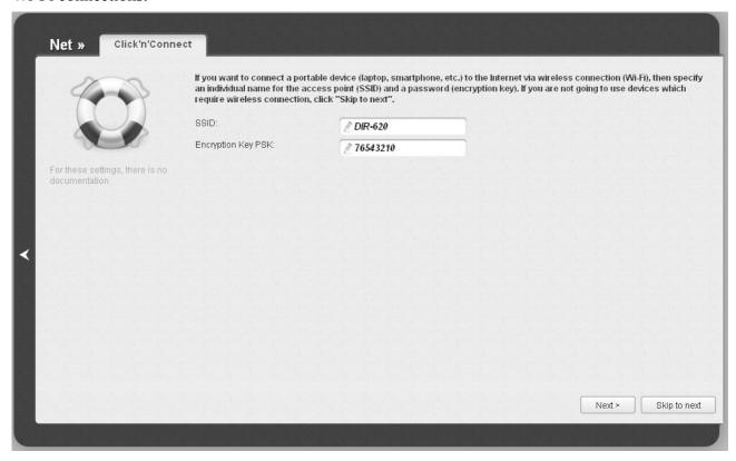
Figure 61. Configuring the wireless connection.
