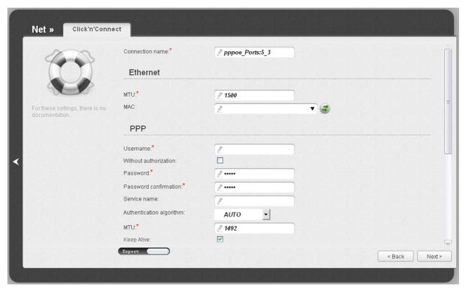
Figure 28. Configuring PPPoE WAN connection. The expert settings mode. The Ethernet section.
