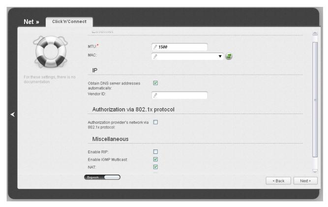
Figure 52. Configuring PPTP + Dynamic IP WAN connection. The expert settings mode. The **IP** and **Authorization via 802.1x protocol** sections.
