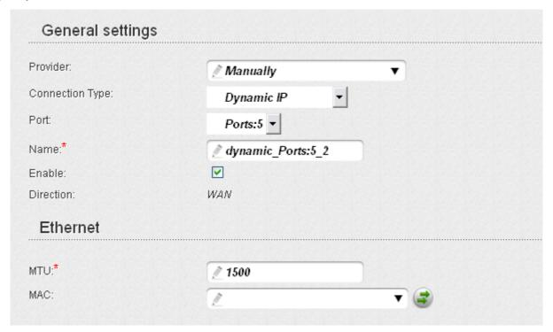
Figure 86. The page for creating a new connection. The **General settings** and **Ethernet** sections.
