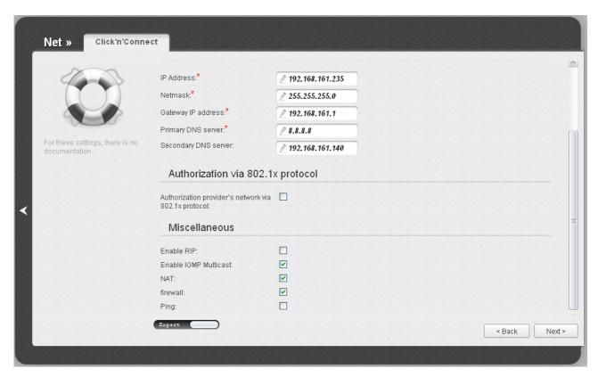
Figure 45. Configuring PPTP + Static IP WAN connection. The expert settings mode. The **Miscellaneous** section.
