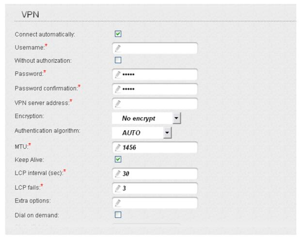
Figure 90. The page for creating a new connection. The **VPN** section.
