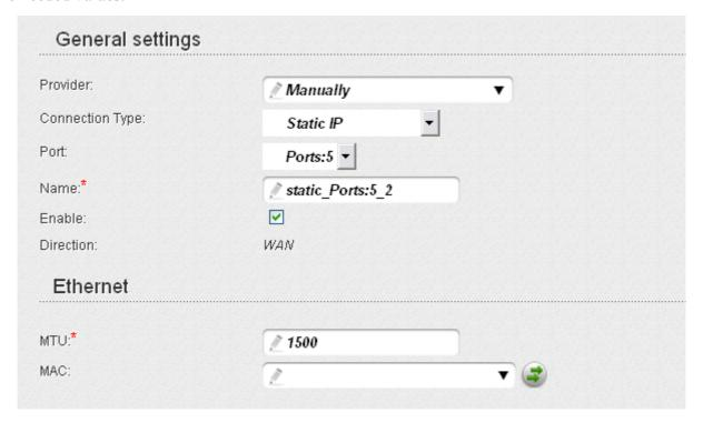
Figure 83. The page for creating a new connection. The **General settings** and **Ethernet** sections.
