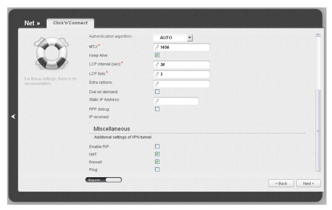
Figure 49. Configuring PPTP + Static IP WAN connection. The expert settings mode. The **Miscellaneous** section.
