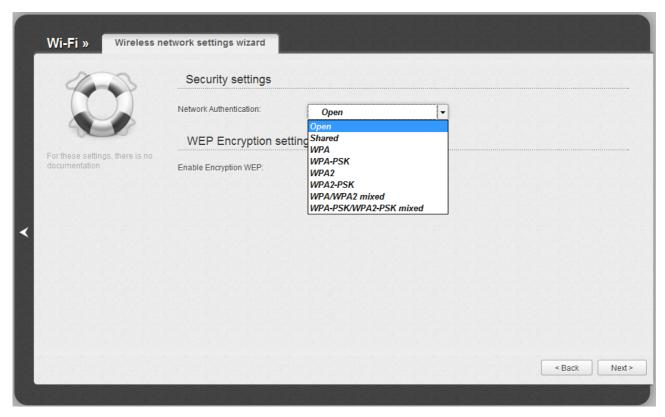
Figure 66. Network authentication types supported by the router.
