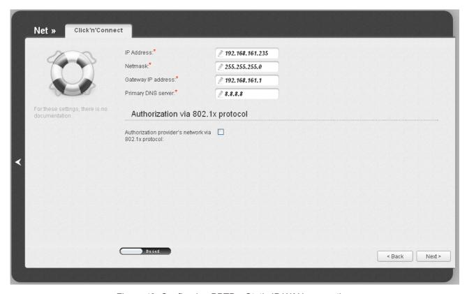
Figure 42. Configuring PPTP + Static IP WAN connection.
