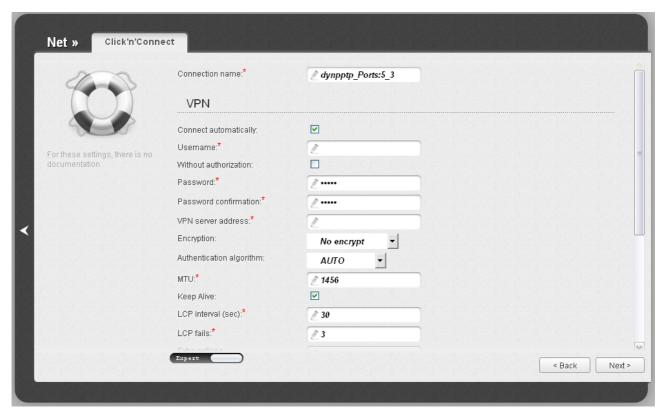
Figure 55. Configuring PPTP + Dynamic IP WAN connection. The expert settings mode. The VPN section.
