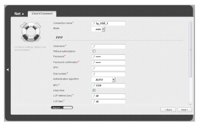
Figure 58. Configuring 3G WAN connection. The expert settings mode. The PPP section.
