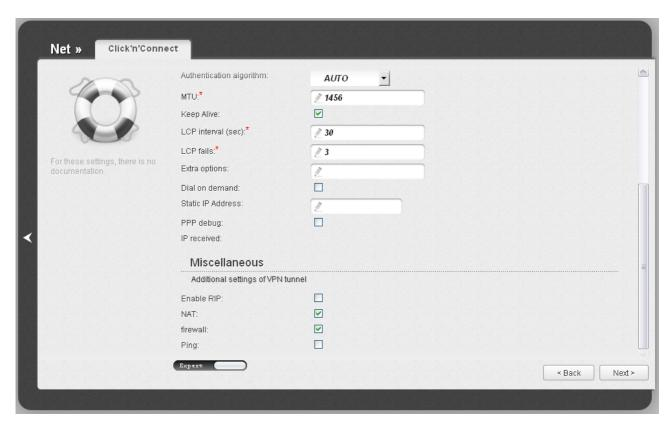
Figure 41. Configuring PPTP WAN connection. The expert settings mode. The Miscellaneous section.
