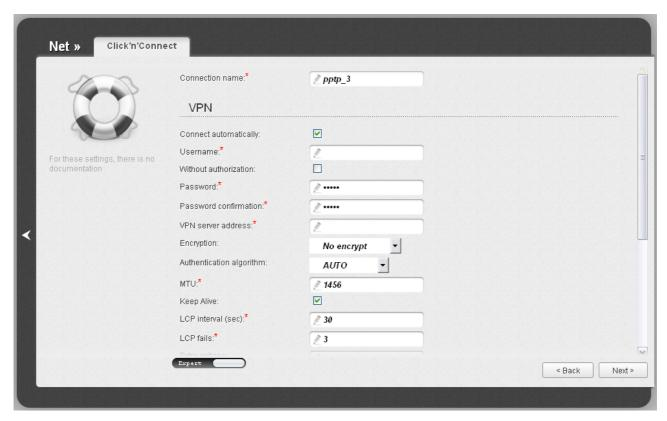
Figure 40. Configuring PPTP WAN connection. The expert settings mode. The VPN section.
