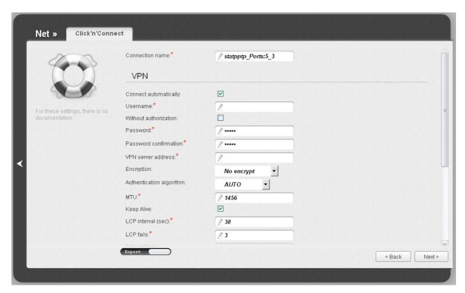
Figure 48. Configuring PPTP + Static IP WAN connection. The expert settings mode. The **VPN** section.
