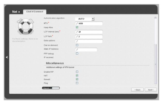
Figure 56. Configuring PPTP + Dynamic IP WAN connection. The expert settings mode. The **Miscellaneous** section.
