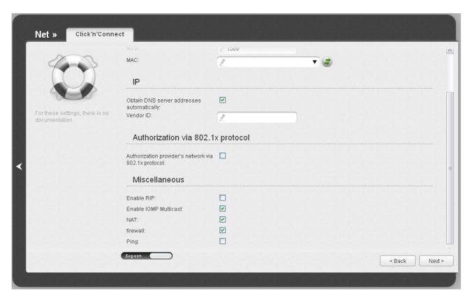
Figure 38. Configuring Dynamic IP WAN connection. The expert settings mode. The Miscellaneous section.
