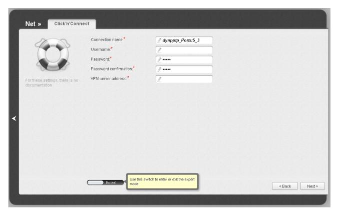
Figure 54. Configuring PPTP + Dynamic IP WAN connection.
