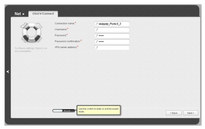
Figure 47. Configuring PPTP + Static IP WAN connection.
