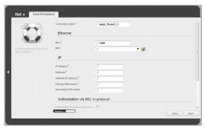
Figure 32. Configuring Static IP WAN connection. The expert settings mode. The Ethernet section.
