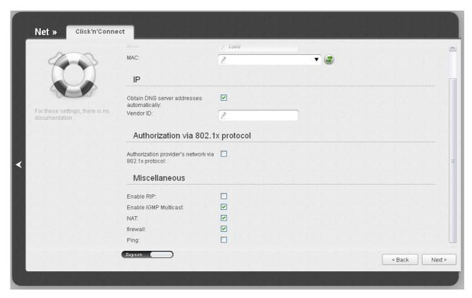
Figure 53. Configuring PPTP + Dynamic IP WAN connection. The expert settings mode. The **Miscellaneous** section.
