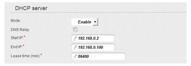
Figure 103. The section for configuring the DHCP server.
