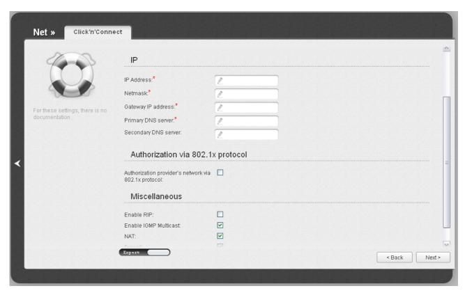
Figure 33. Configuring Static IP WAN connection. The expert settings mode. The **IP** and **Authorization via 802.1x protocol** sections.
