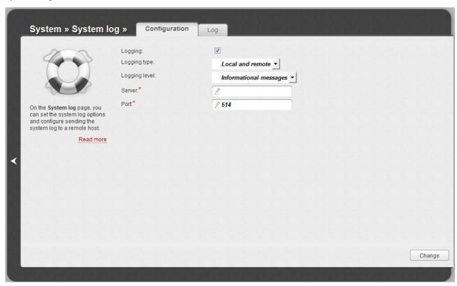
Figure 152. The **System / System log** page. The **Configuration** tab.
