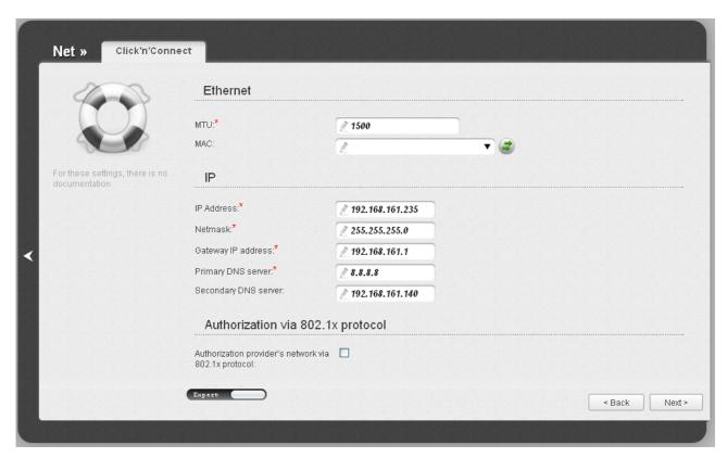
Figure 43. Configuring PPTP + Static IP WAN connection. The expert settings mode. The **Ethernet** section.
