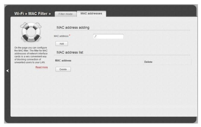
Figure 113. The tab for adding a MAC address.
