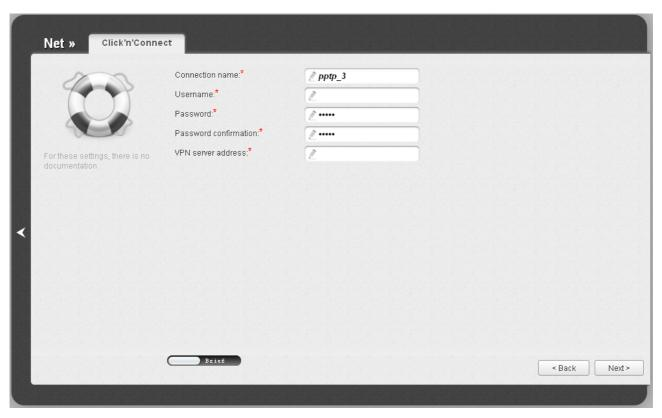
Figure 39. Configuring PPTP WAN connection.
