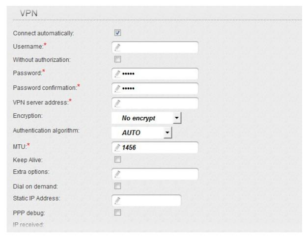
Figure 100. The page for creating a new connection. The **VPN** section.
