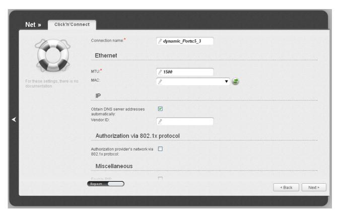
Figure 36. Configuring Dynamic IP WAN connection. The expert settings mode. The **Ethernet** section.
