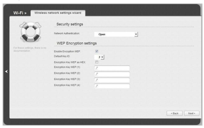
Figure 67. The Open value is selected from the Network Authentication drop-down list.
