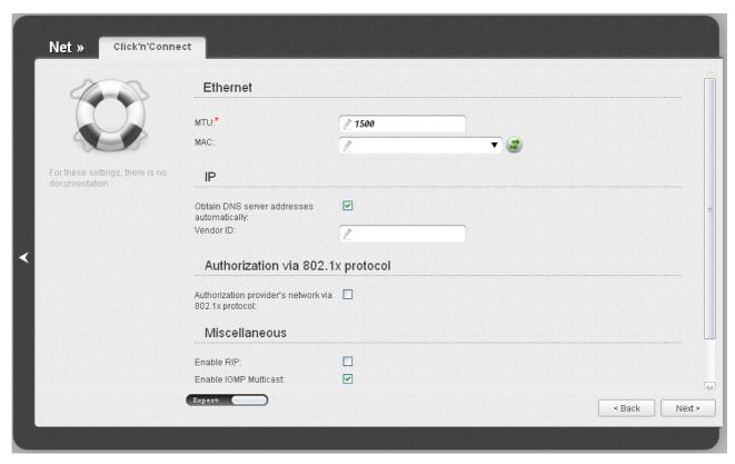
Figure 51. Configuring PPTP + Dynamic IP WAN connection. The expert settings mode. The **Ethernet** section.
