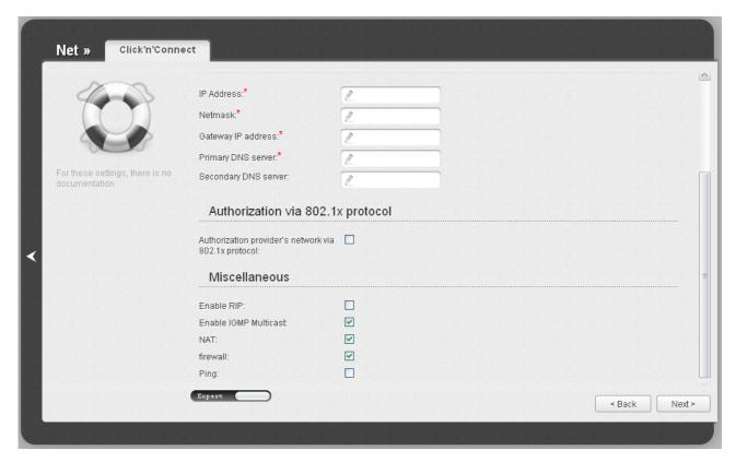
Figure 34. Configuring Static IP WAN connection. The expert settings mode. The Miscellaneous section.
