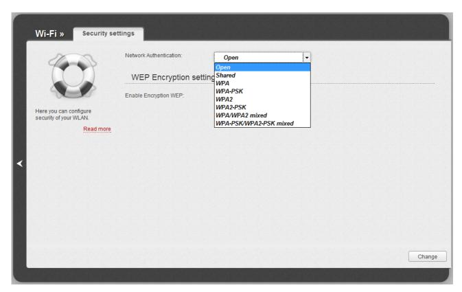
Figure 108. Network authentication types supported by the router.
