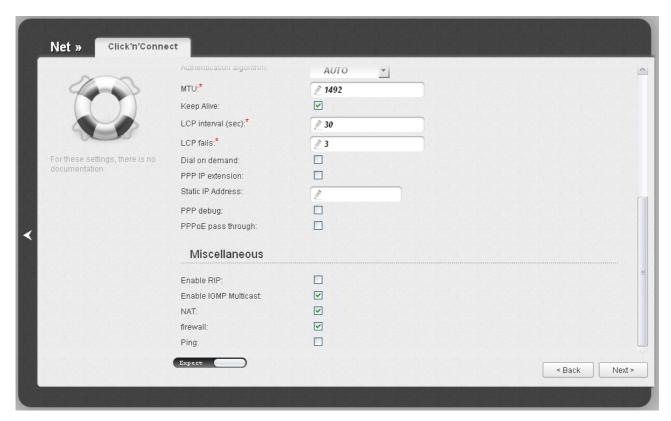
Figure 30. Configuring PPPoE WAN connection. The expert settings mode. The Miscellaneous section.
