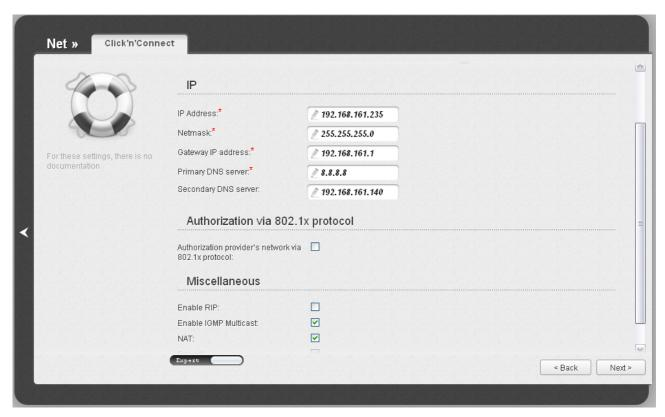
Figure 44. Configuring PPTP + Static IP WAN connection. The expert settings mode. The **IP** and **Authorization via 802.1x protocol** sections.
