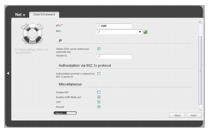
Figure 37. Configuring Dynamic IP WAN connection. The expert settings mode. The **IP** and **Authorization** via 802.1x protocol sections.
