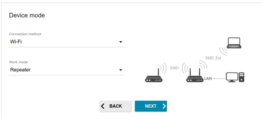
Figure 37. Selecting an operation mode. The **Repeater** mode.
