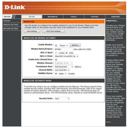
**Enable Auto** The **Auto Channel Scan** setting can be selected to allow the DIR-628 to choose the channel with the least amount of interference.
