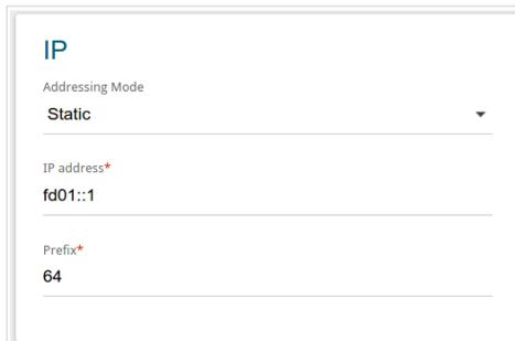
The screenshot shows the IPv6 configuration page. At the top, there is a tab labeled "IPv6". Below the tab, the section is titled "IP". There are three input fields: "Addressing Mode" with a dropdown menu showing "Static", "IP address\*" with the value "fd01::1", and "Prefix\*" with the value "64".
