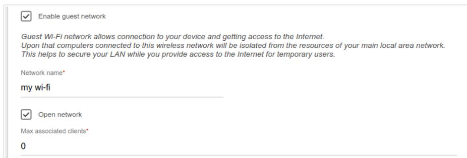
Figure 40. The page for configuring the wireless network.
