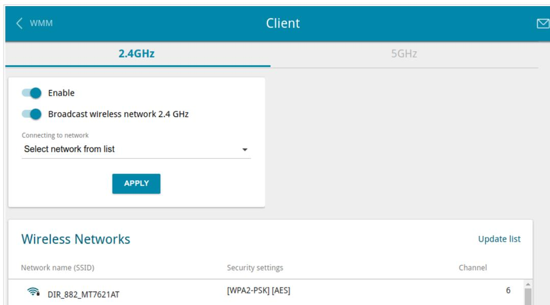
Figure 91. The page for configuring the client mode.
