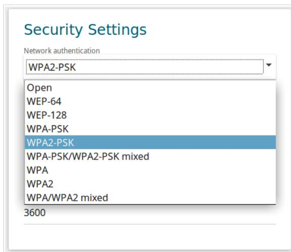
Figure 83. Network authentication types supported by the router.
