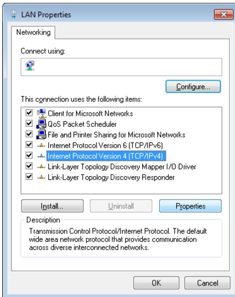
Figure 9. The **Local Area Connection Properties** window.
