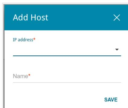
Figure 101. The window for adding a DNS record.
