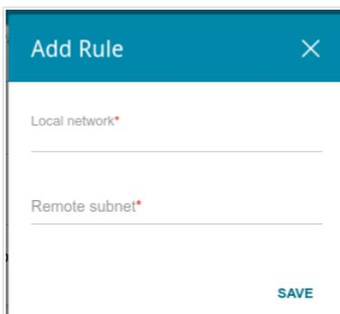
Figure 119. The page for adding an IPsec tunnel. The window for adding a tunneled network.
