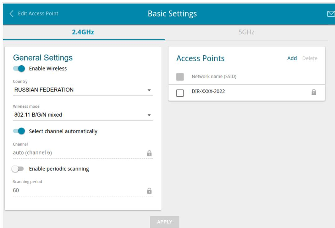
Figure 81. Basic settings of the wireless LAN in the 2.4GHz band.
