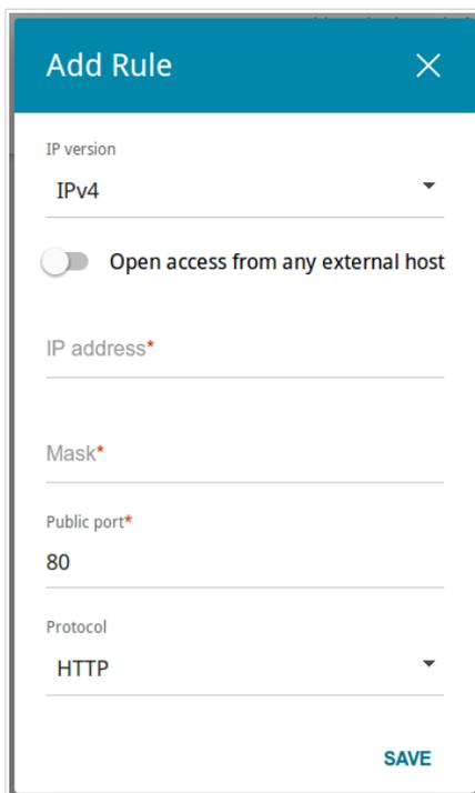
Figure 111. The window for adding a rule for remote management.
