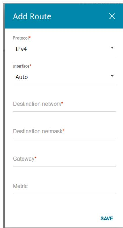
The 'Add Route' window is a vertical form with a teal header containing the title 'Add Route' and a close 'X' button. The form contains several input fields: 'Protocol\*' with a dropdown menu showing 'IPv4'; 'Interface\*' with a dropdown menu showing 'Auto'; 'Destination network\*'; 'Destination netmask\*'; 'Gateway\*'; and 'Metric'. A teal 'SAVE' button is located at the bottom right of the form.
