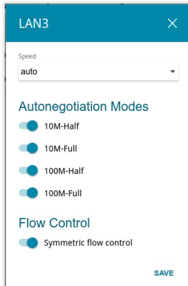
Figure 103. The window for changing the settings of the router's port.
