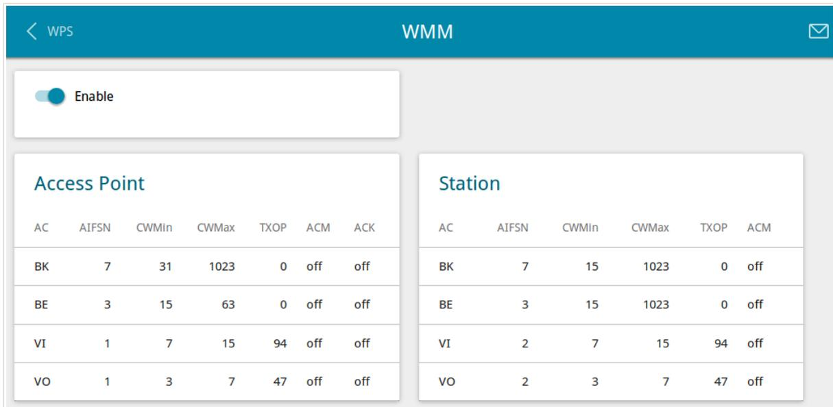
Figure 89. The page for configuring the WMM function.
