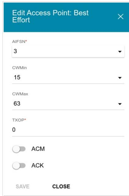
Figure 96. The window for changing parameters of the WMM function.
