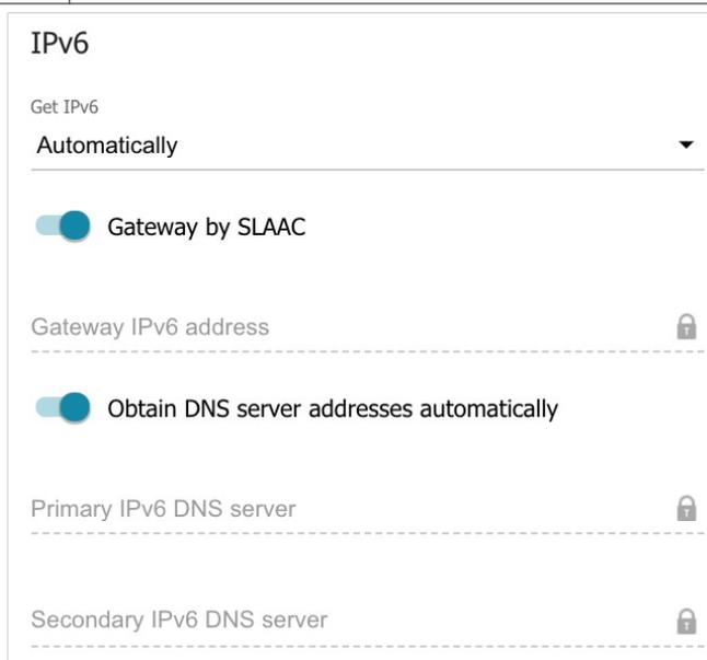
Figure 77. The page for creating a new PPPoE Pv6 connection. The IPv6 section.
