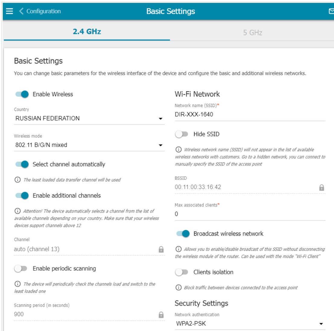
Figure 87. General settings of the wireless connection in the 2.4GHz band.
