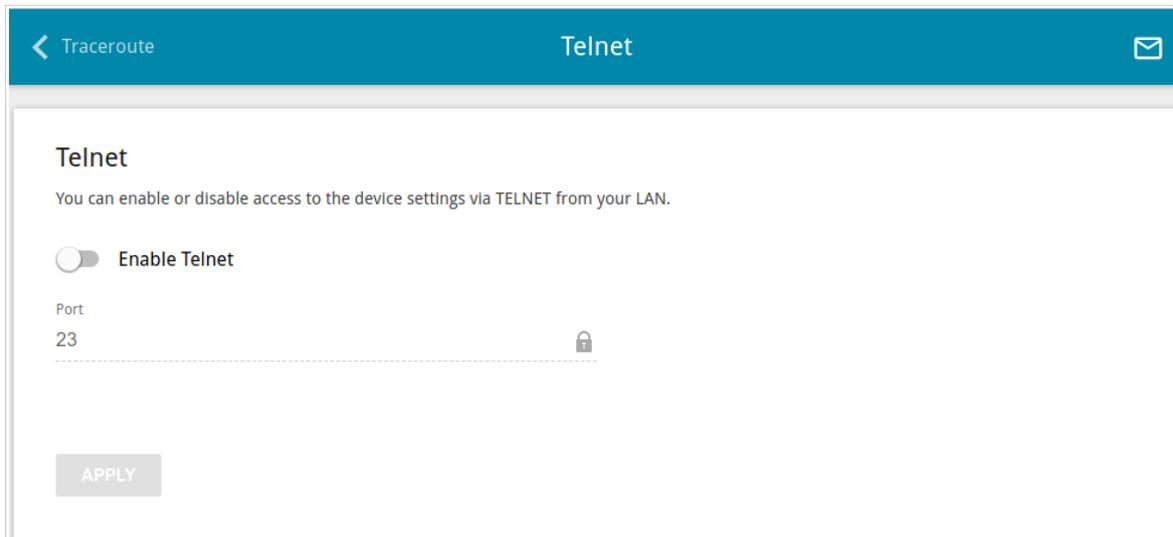
Figure 143. The **System / Telnet** page.
