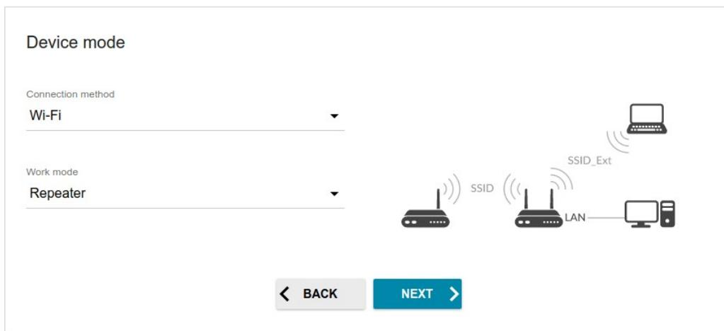
Figure 36. Selecting an operation mode. The **Repeater** mode.
