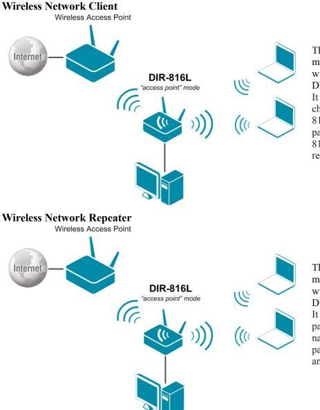
The DIR-816L device in the "access point" mode is connected to an access point via wireless connection. Computers connect to DIR-816L via wireless or wired connection. It is necessary to configure the same channel of the wireless connection for DIR-816L and the remote access point. Other parameters of the wireless network of DIR-816L do not depend upon the settings of the remote access point.
