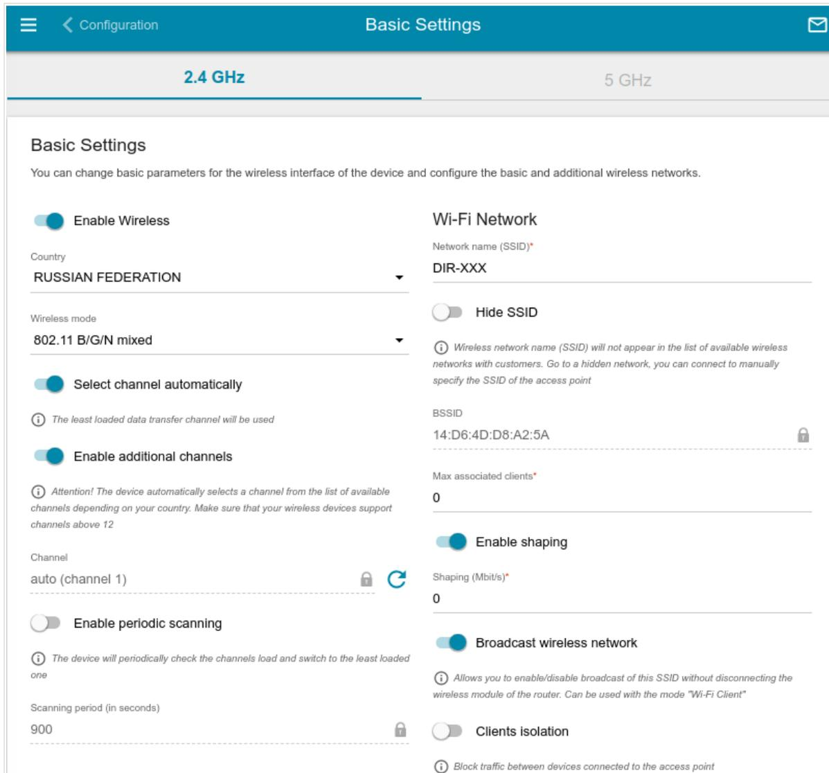
Figure 97. General settings of the wireless connection in the 2.4GHz band.
