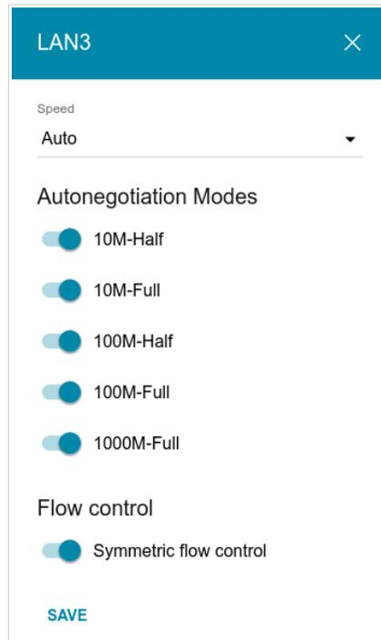
Figure 140. The window for changing the settings of the router's port.
