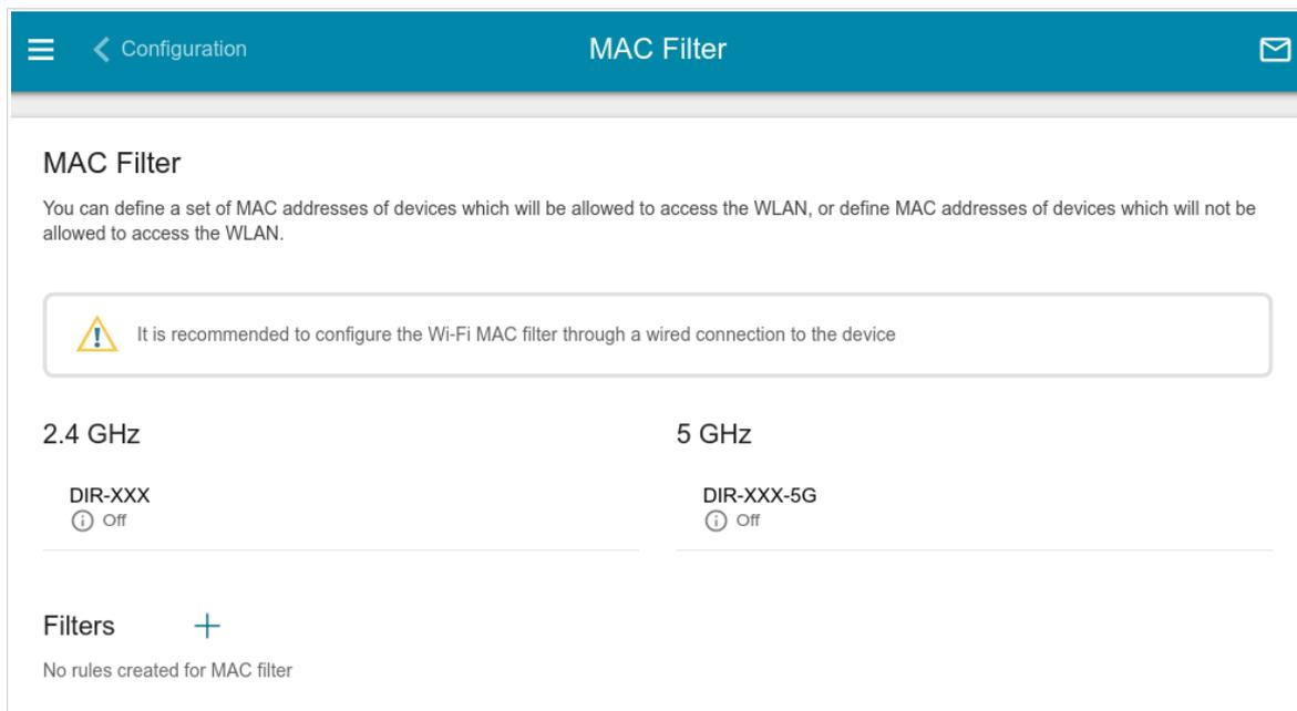
Figure 111. The page for configuring the MAC filter for the wireless network.
