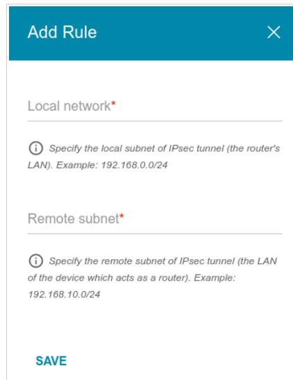
Figure 158. The page for adding an IPsec tunnel. The window for adding a tunneled network.
