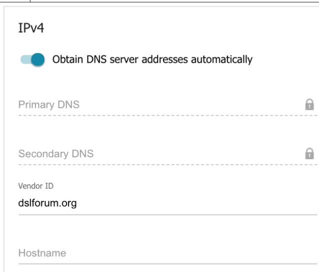
Figure 87. The page for creating a new **LTE** connection. The **IPv4** section.
