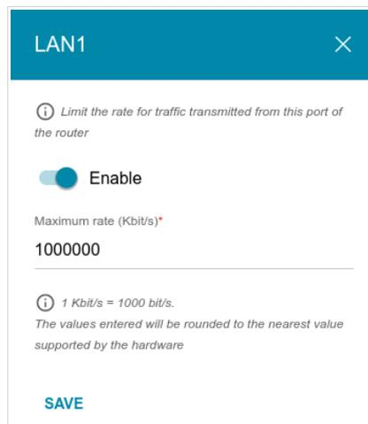
Figure 142. The window for setting up rate limit.
