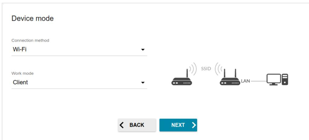
Figure 38. Selecting an operation mode. The **Client** mode.
