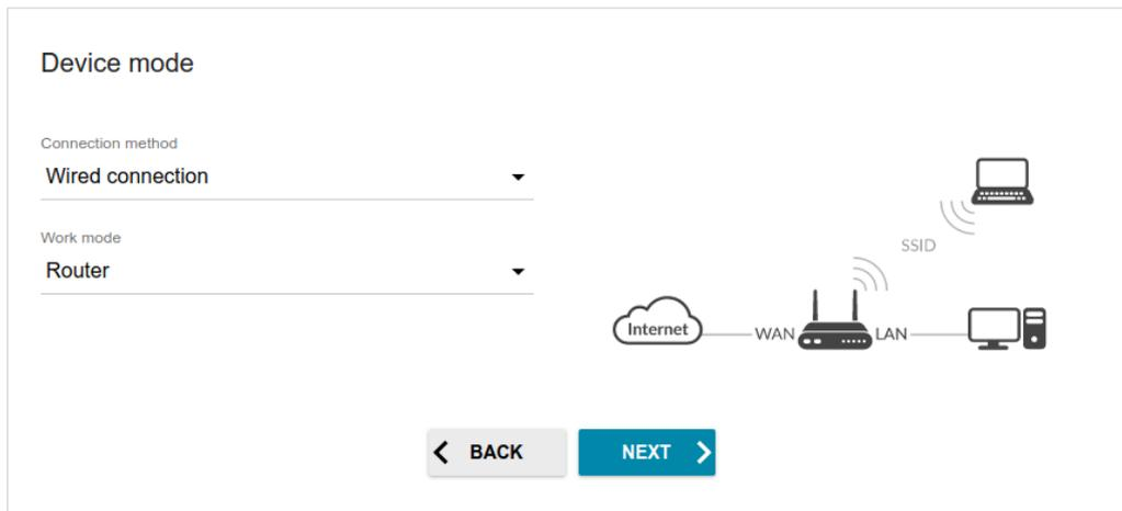
Figure 33. Selecting an operation mode. The **Router** mode.
