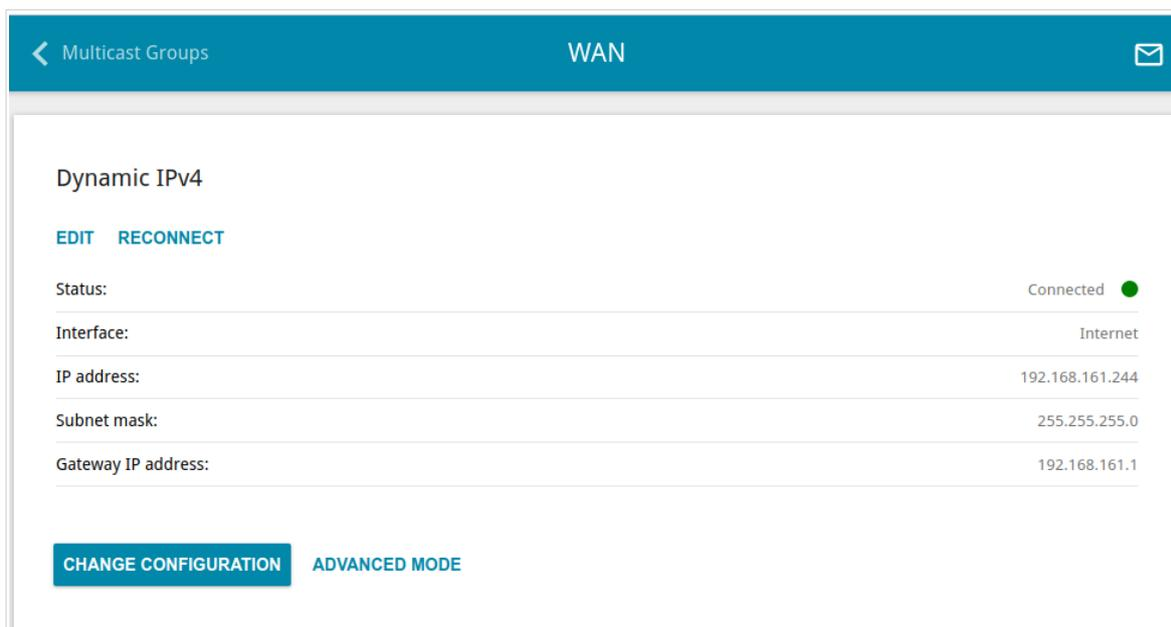
Figure 64. The **Connections Setup / WAN** page. The simplified mode.
