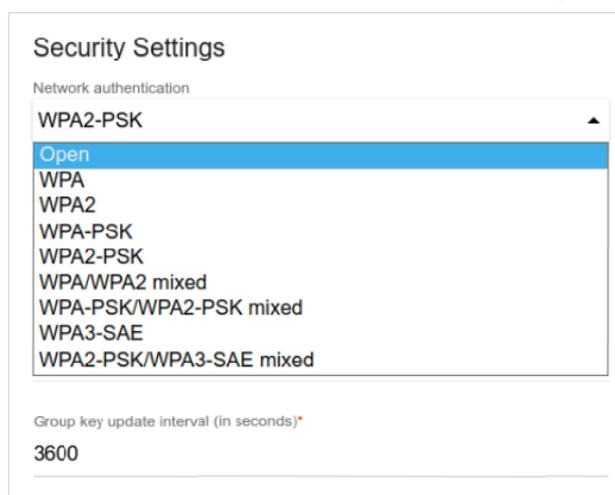
Figure 99. Network authentication types supported by the router.
