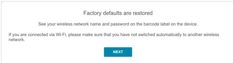
If you perform initial configuration of the router via Wi-Fi connection, please make sure that you are connected to the wireless network of DIR-825 (see the WLAN name (SSID) in the **Default Settings** section, page 3) and click the **NEXT** button. Then click the **START** button.
