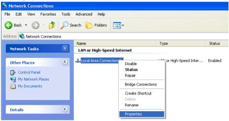
In the Local Area Connection Properties window, on the General tab, select the Internet Protocol (TCP/IP) line. Click the Properties button. 4. Select the **Obtain an IP address automatically** and **Obtain DNS server address automatically** radio buttons. Click the **OK** button.
