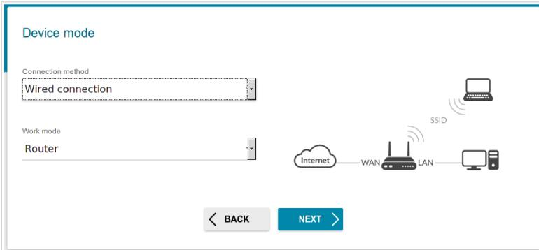
In order to connect your device to the network of a 3G or LTE operator, on the **Device mode** page, from the **Connection method** list, select the **3G/LTE modem** value. In this mode you can configure a 3G/LTE WAN connection, set your own settings for the wireless network, and set your own password for access to the web-based interface of the device.
