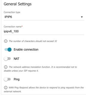
Figure 85. The page for creating a new **IPIP6** connection. The **General Settings** section.
