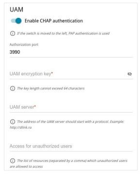
Figure 157. The page for adding an authorization server. The UAM section.
