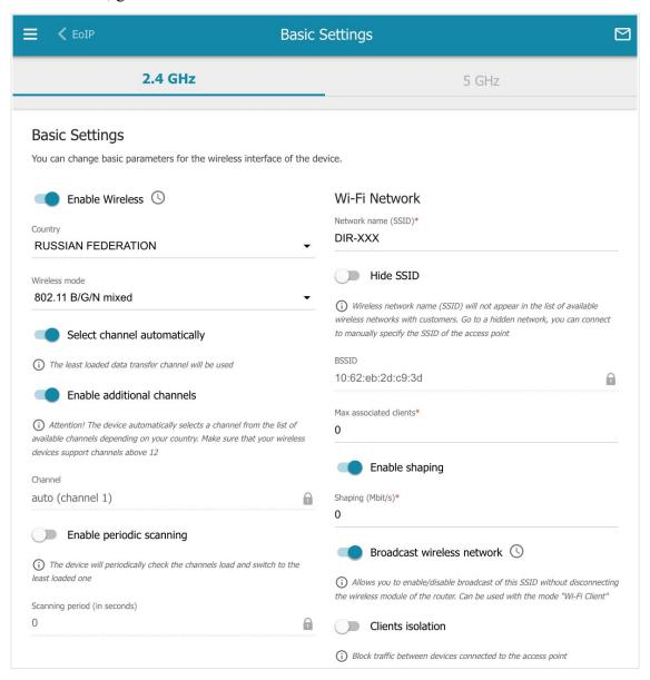
Figure 121. Basic settings of the wireless LAN in the 2.4GHz band.
