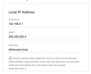
Figure 93. Configuring the local interface. The IPv4 tab. The Local IP Address section.
