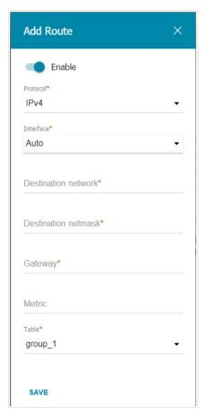
Figure 145. The window for adding a new route.
