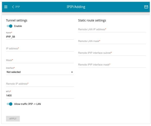
Figure 112. The page for adding an IPIP tunnel.
