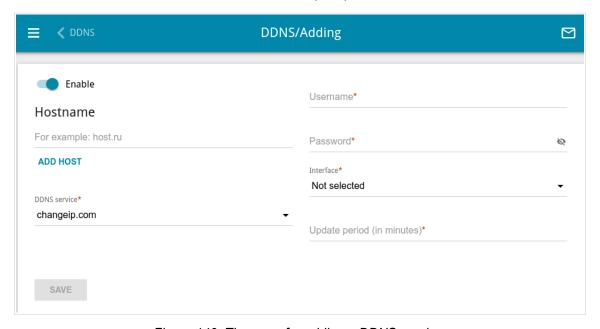
Figure 140. The page for adding a DDNS service.
