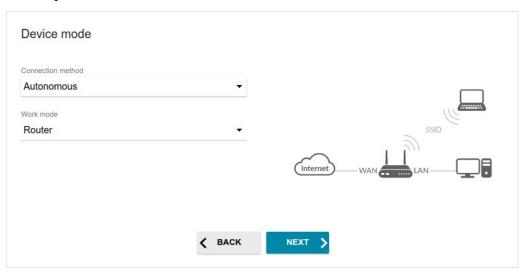
Figure 33. Selecting an operation mode. The Router mode.
