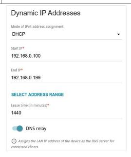
Figure 94. Configuring the local interface. The **IPv4** tab. The **Dynamic IP Addresses** section.
