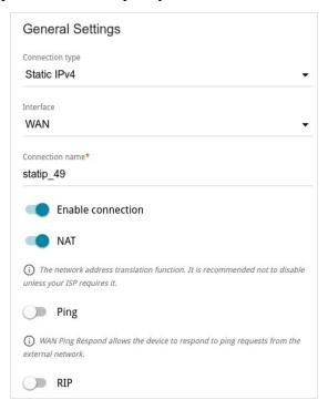
Figure 69. The page for creating a new Static IPv4 connection. The General Settings section.
