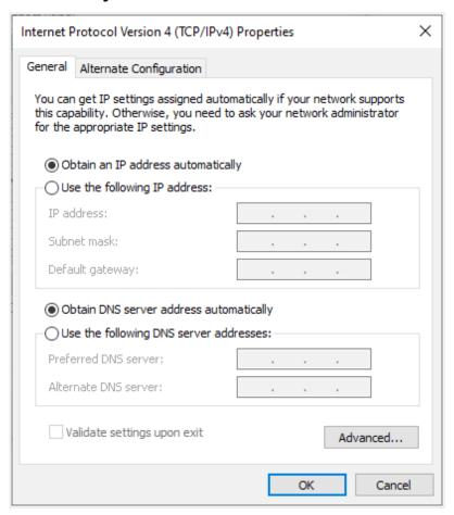
Figure 18. The Internet Protocol Version 4 (TCP/IPv4) Properties window.
