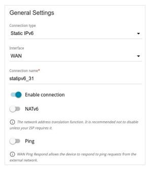
Figure 72. The page for creating a new **Static IPv6** connection. The **General Settings** section.
