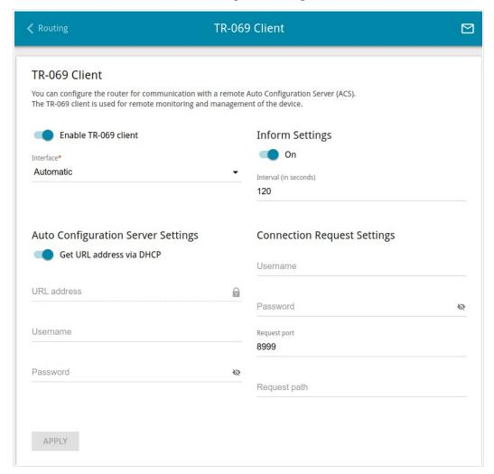
Figure 146. The page for configuring the TR-069 client.
