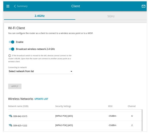
Figure 129. The page for configuring the client mode.
