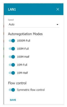
Figure 142. The window for changing the settings of the router's port.
