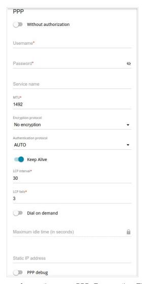
Figure 77. The page for creating a new **PPPoE** connection. The **PPP** section.
