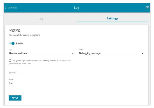
Figure 177. The System / Log page. The Settings tab.
