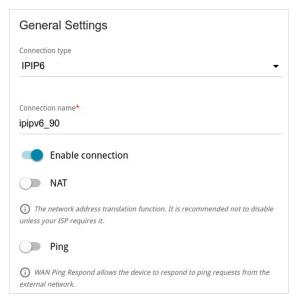
Figure 88. The page for creating a new IPIP6 connection. The General Settings section.
