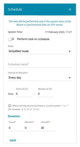
Figure 176. The window for adding a schedule for a task.
