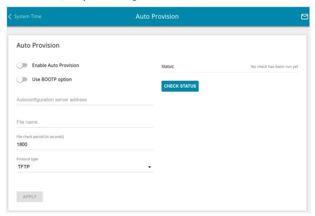
Figure 185. The page for configuring the Auto Provision function.
