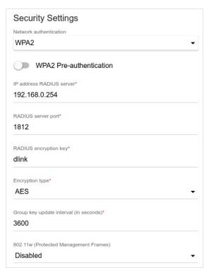
Figure 126. The WPA2 value is selected from the Network authentication drop-down list.
