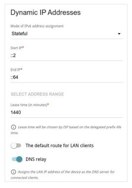
Figure 100. Configuring the local interface. The IPv6 tab. The Dynamic IP Addresses section.
