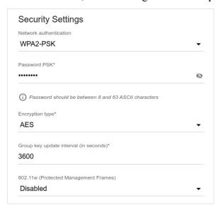
Figure 125. The WPA2-PSK value is selected from the Network authentication drop-down list.
