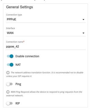
Figure 75. The page for creating a new **PPPoE** connection. The **General Settings** section.
