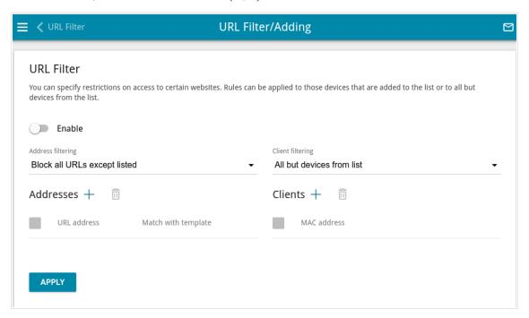
Figure 166. The page for adding a rule for URL filter.
