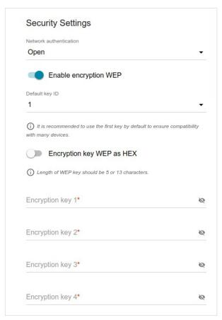
Figure 124. The Open value is selected from the Network authentication drop-down list.
