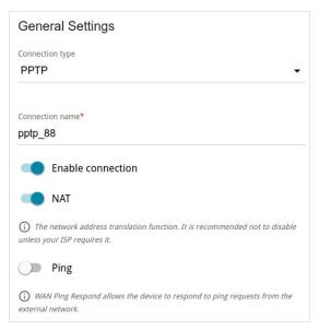
Figure 79. The page for creating a new **PPTP** connection. The **General Settings** section.
