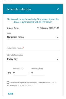
Figure 175. The window for configuring automatic reboot on a schedule.
