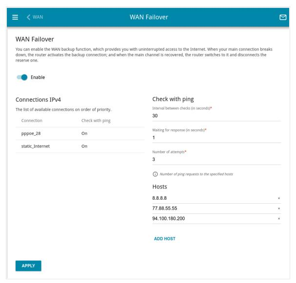
Figure 103. The Connections Setup / WAN Failover page.
