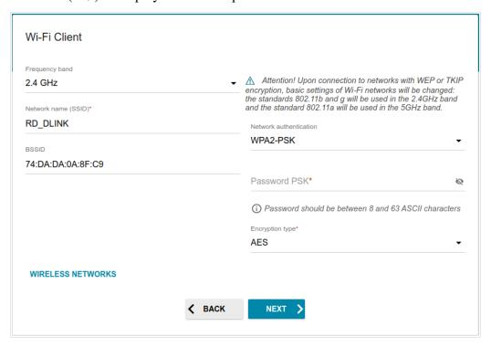
Figure 42. The page for configuring the Wi-Fi client.
