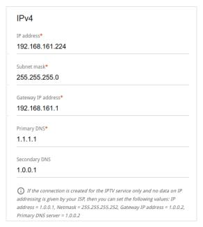
Figure 71. The page for creating a new Static IPv4 connection. The IPv4 section.
