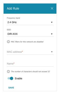
Figure 132. The window for adding a rule for the MAC filter.
