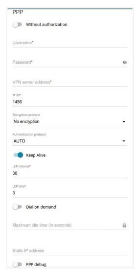
Figure 80. The page for creating a new PPTP connection. The PPP section.
