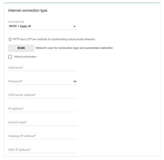
Figure 48. The page for configuring PPTP + Static IP WAN connection.
