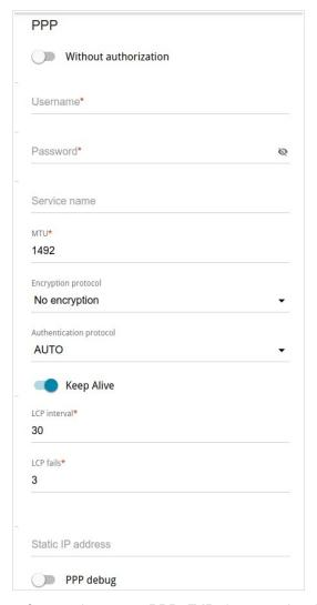
Figure 85. The page for creating a new **PPPoE IPv6** connection. The **PPP** section.
