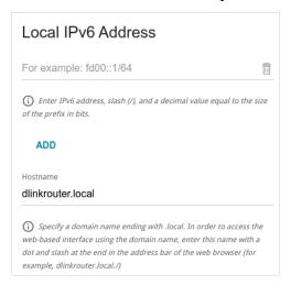
Figure 99. Configuring the local interface. The IPv6 tab. The Local IPv6 Address section.
