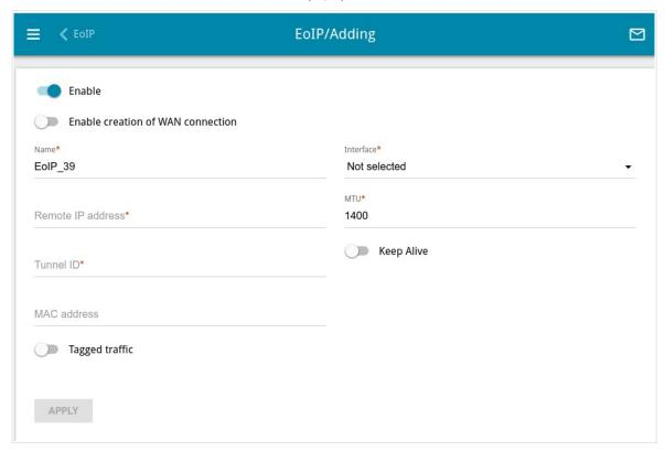
Figure 120. The page for adding an EoIP tunnel.
