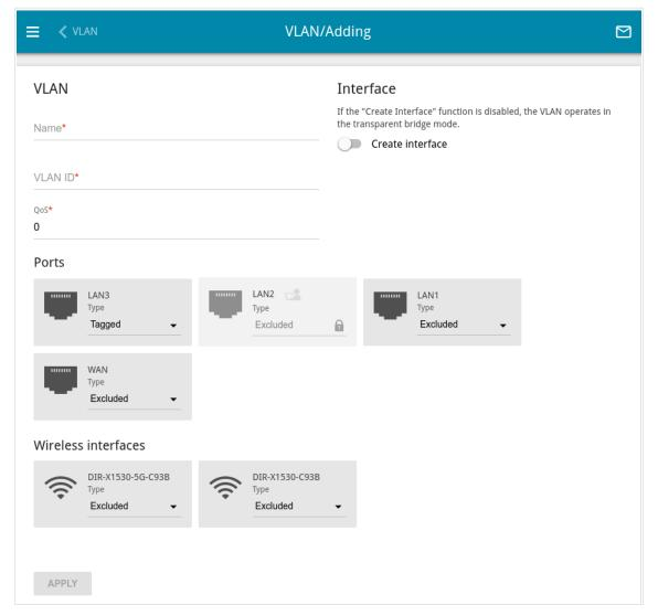
Figure 136. The page for adding a VLAN.
