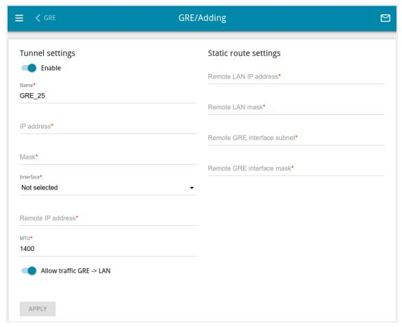
Figure 110. The page for adding a GRE tunnel.
