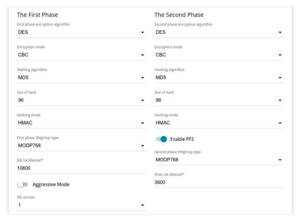
Figure 107. The page for adding an IPsec tunnel. The First Phase / The Second Phase sections.
