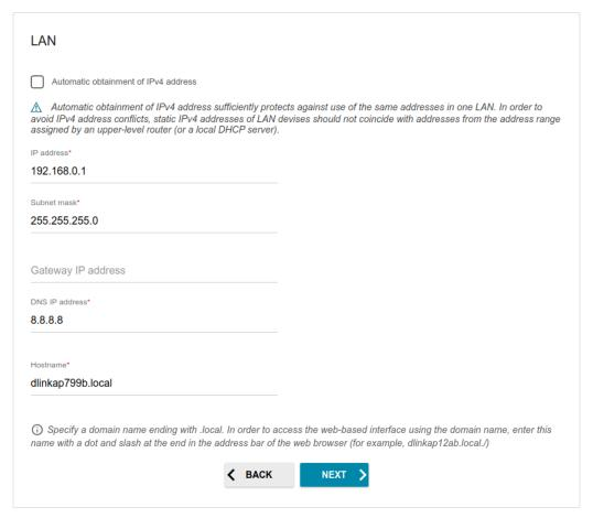
Figure 41. The page for changing the LAN IPv4 address.
