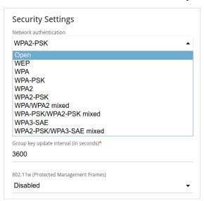
Figure 123. Network authentication types supported by the router.
