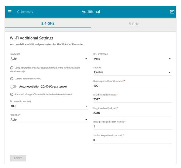
Figure 130. Additional settings of the WLAN.
