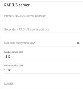
Figure 155. The page for adding an authorization server. The **RADIUS server** section.
