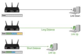
D-Link Green Ethernet detects link status and cable length and adjusts power usage accordingly.
