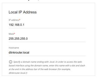
Figure 90. Configuring the local interface. The IPv4 tab. The Local IP Address section.
