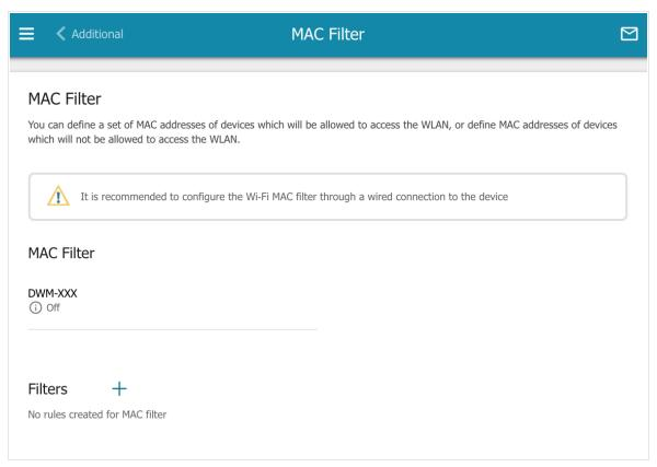
Figure 133. The page for configuring the MAC filter for the wireless network.
