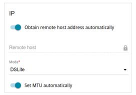
Figure 86. The page for creating a new **IPIP6** connection. The **IP** section.
