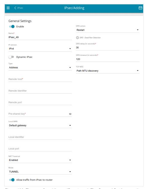
Figure 106. The page for adding an IPsec tunnel. The General Settings section.
