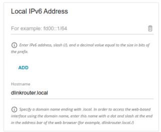
Figure 96. Configuring the local interface. The IPv6 tab. The Local IPv6 Address section.
