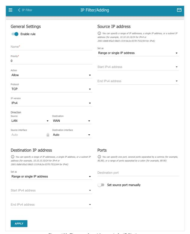
Figure 163. The page for adding a rule for IP filtering.
