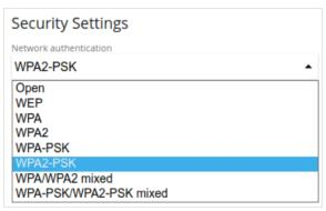
Figure 123. Network authentication types supported by the router.
