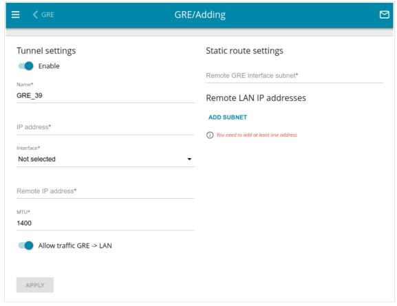
Figure 110. The page for adding a GRE tunnel.
