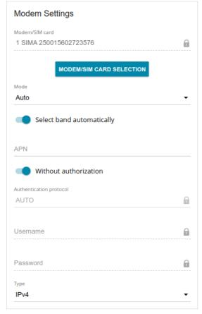
Figure 81. The page for creating a new Mobile Internet connection. The Modem Settings section.
