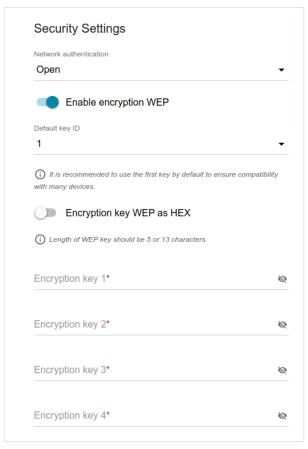
Figure 124. The **Open** value is selected from the **Network authentication** drop-down list.
