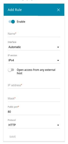
Figure 171. The window for adding a rule for remote management.
