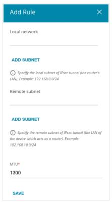
Figure 108. The page for adding an IPsec tunnel. The window for adding a tunneled network.
