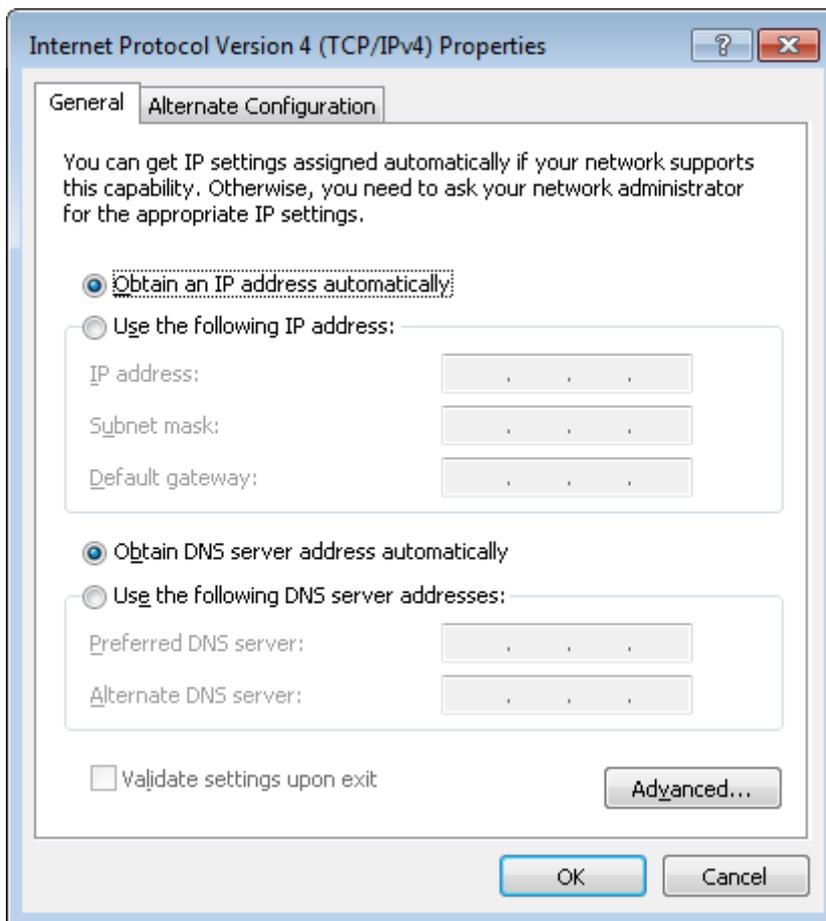
Figure 7. The **Internet Protocol Version 4 (TCP/IPv4) Properties** window.
