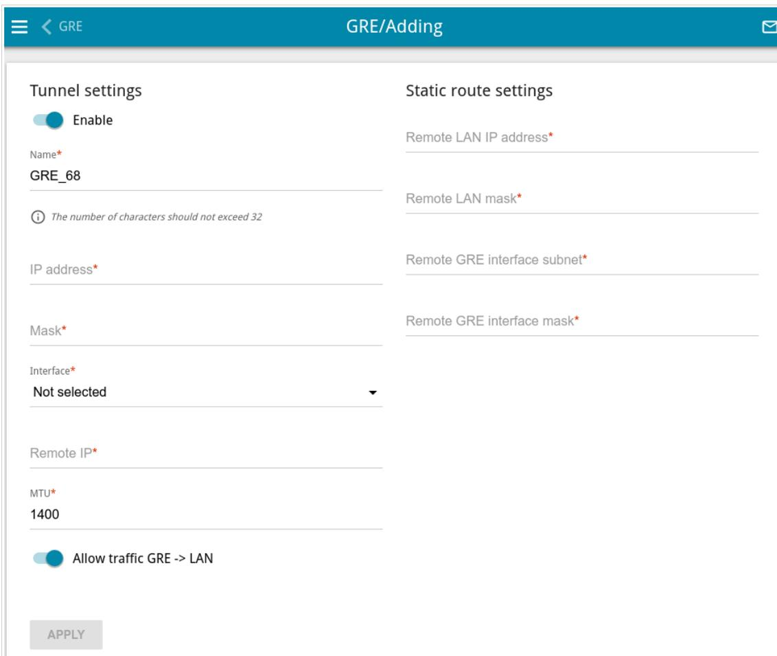
Figure 116. The page for adding a GRE tunnel.
