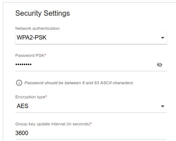
Figure 123. The **WPA2-PSK** value is selected from the **Network authentication** drop-down list.
