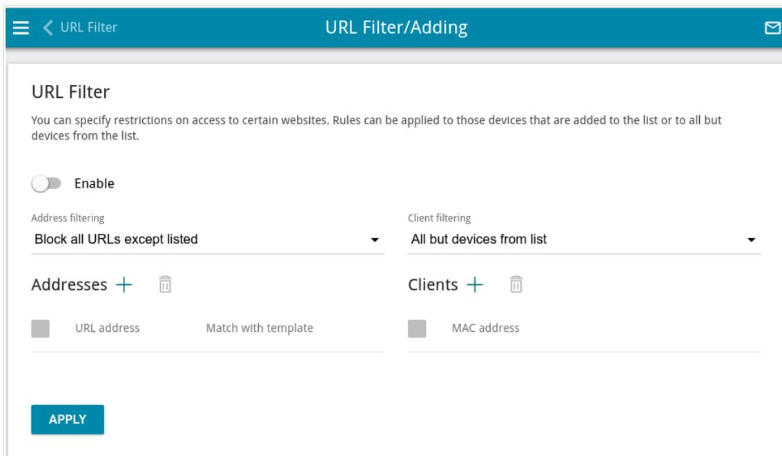
Figure 167. The page for adding a rule for URL filter.
