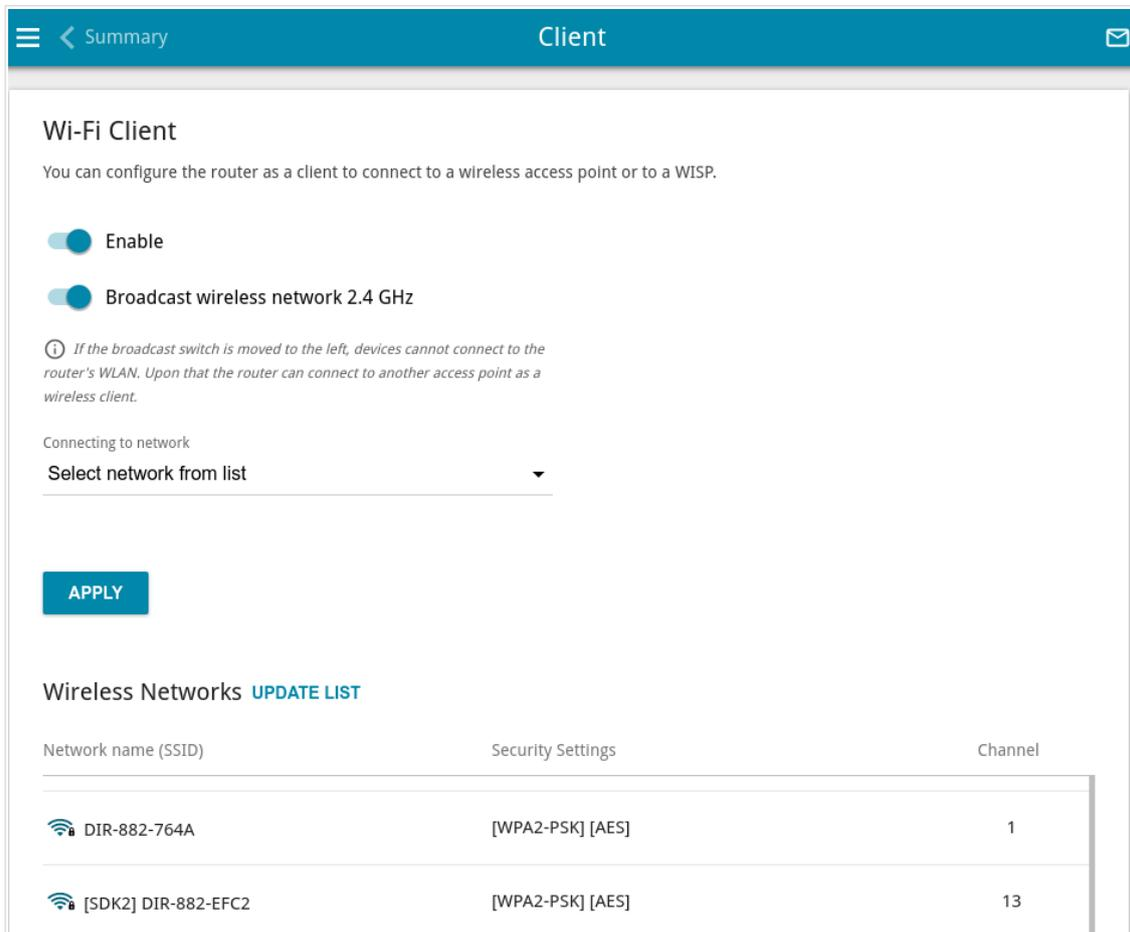
Figure 129. The page for configuring the client mode.
