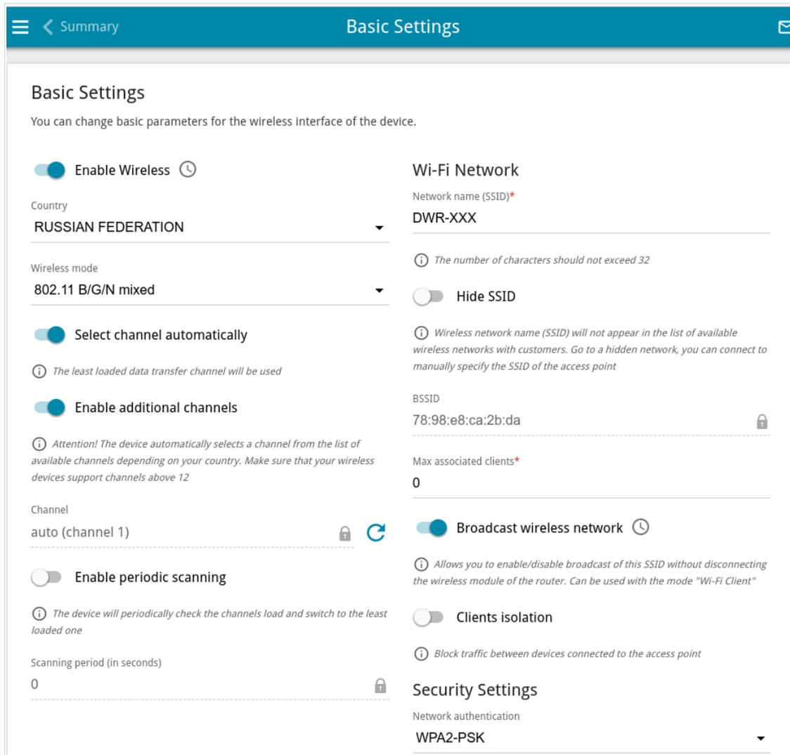
Figure 119. Basic settings of the wireless LAN.
