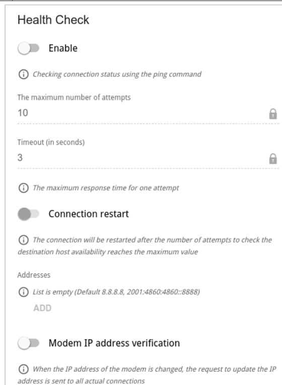
Figure 92. The page for creating a new **Mobile Internet** connection. The **Health Check** section.
