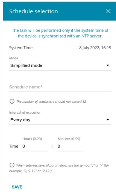
Figure 175. The window for configuring automatic reboot on a schedule.
