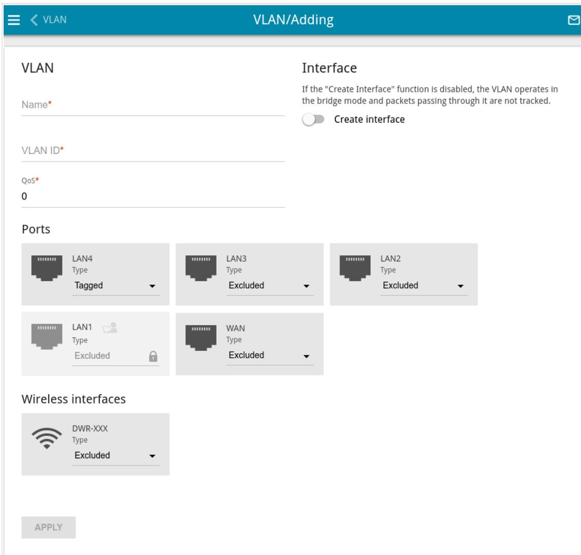
Figure 142. The page for adding a VLAN.
