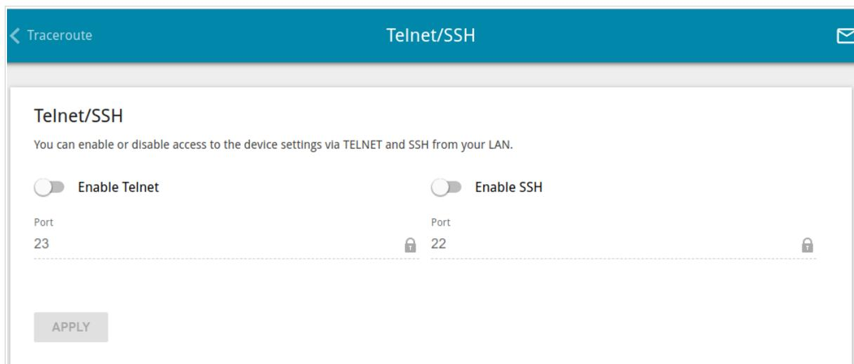
Figure 183. The **System / Telnet/SSH** page.
