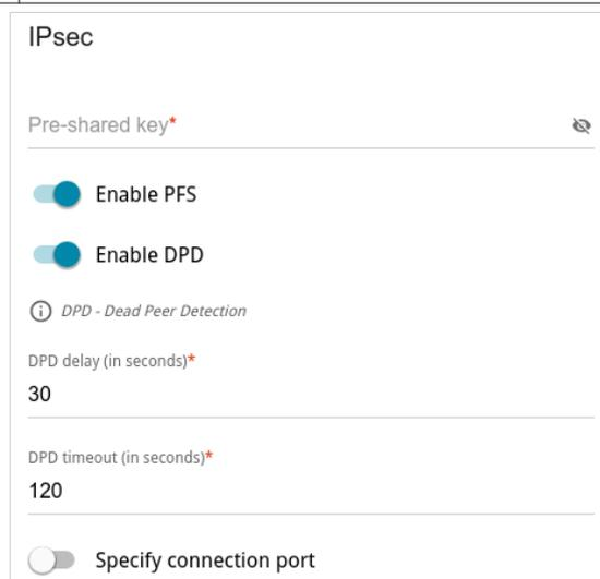
Figure 82. The page for creating a new **L2TP over IPsec** connection. The **IPsec** section.
