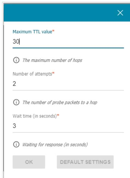
Figure 182. The **System / Traceroute** page. The additional settings window.
