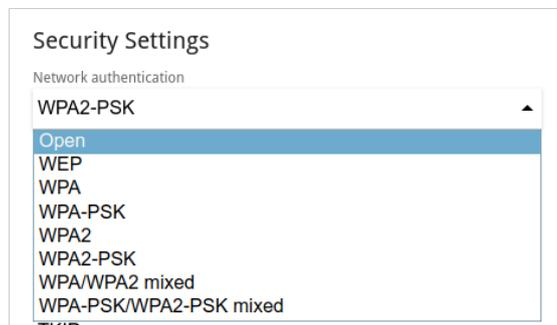
Figure 121. Network authentication types supported by the router.
