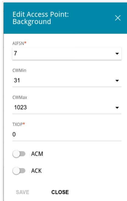
Figure 128. The window for changing parameters of the WMM function.
