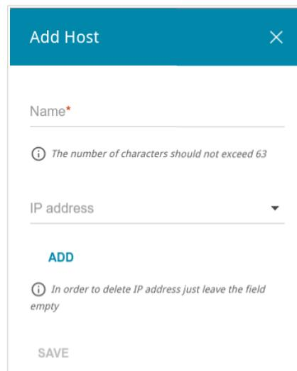
Figure 107. Configuring the local interface. The IPv6 tab. The window for adding a DNS record.
