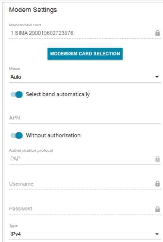
Figure 89. The page for creating a new **Mobile Internet** connection. The **Modem Settings** section.
