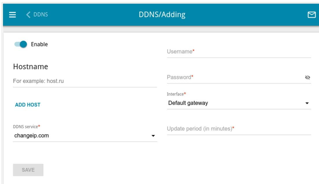
Figure 146. The page for adding a DDNS service.
