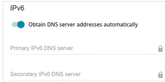
Figure 91. The page for creating a new **Mobile Internet** connection. The **IPv6** section.
