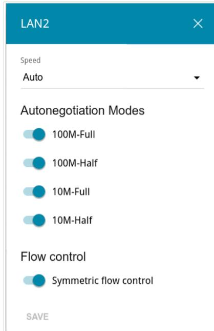
Figure 148. The window for changing the settings of the router's port.
