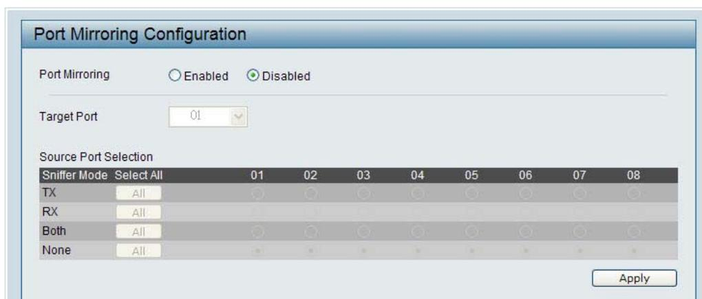
**Figure 31. Configuration > Port Mirroring**
