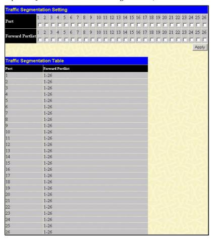
Figure 6-50. Traffic Segmentation Setting window
