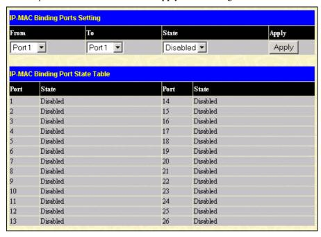
Figure 6-83. IP-MAC Binding Ports window
