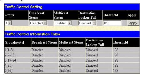
Figure 6-43. Traffic Control Setting window
