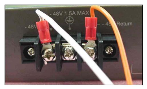
Figure 2-4. Power connections attached to contacts on assembly
