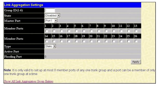
Figure 6- 10. Link Aggregation Settings window - Modify
