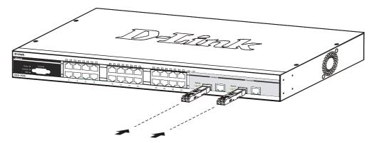
Figure 1-7. Mini-GBIC modules plug-in to the Switch
