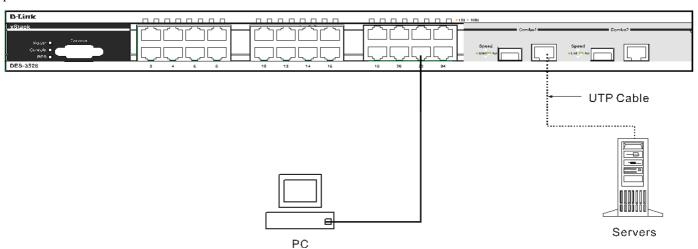
Figure 3- 3. Connecting the DES-3526 to a Server
