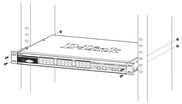
Figure 2-3. Installing Switch in a rack
