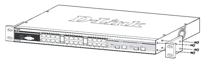
Figure 2- 2. Fasten mounting brackets to Switch
