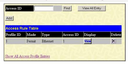
Figure 6- 63. Access Rule Table window (Ethernet)
