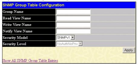
Figure 7-35. SNMP Group Table Configuration window
