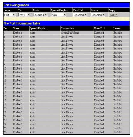
Figure 6-4. Port Configuration window
