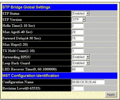
Figure 6-21. STP Bridge Global Settings window - STP
