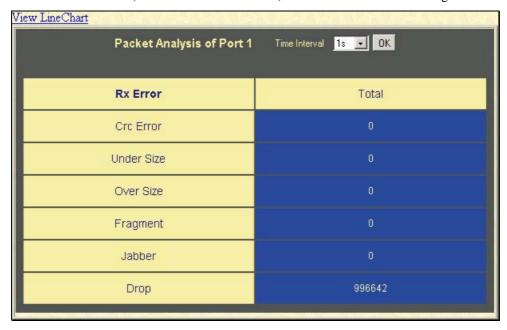
Figure 8- 10. Rx Error Analysis window (table)
