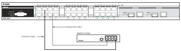
Figure 3- 2. Switch connected to a normal (non-Uplink) port on a hub or switch using a straight or crossover cable
