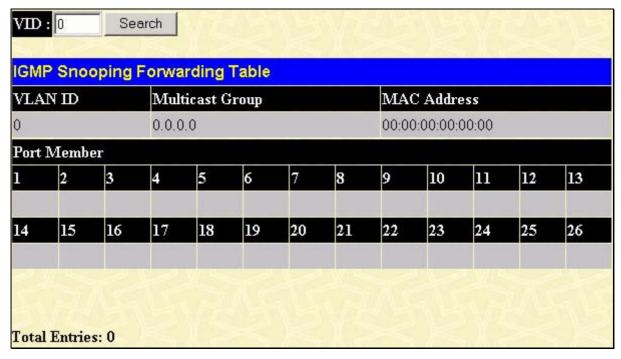
Figure 8-18. IGMP Snooping Forwarding Table window
