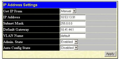
Figure 6-2. IP Address Settings window
