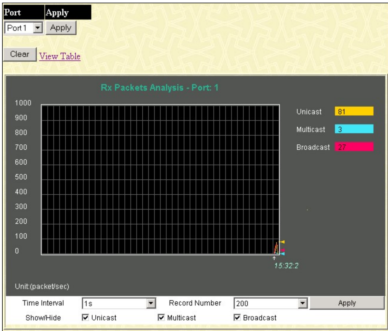
Figure 12- 7. Rx Packets Analysis window (line graph for Unicast, Multicast, and Broadcast Packets)
